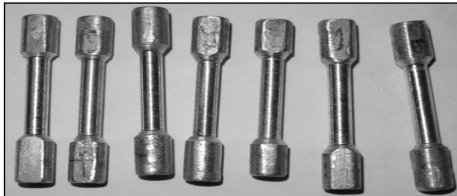
Fig. 4.12 Tensile test pieces machined from sinter-forged briquettes
