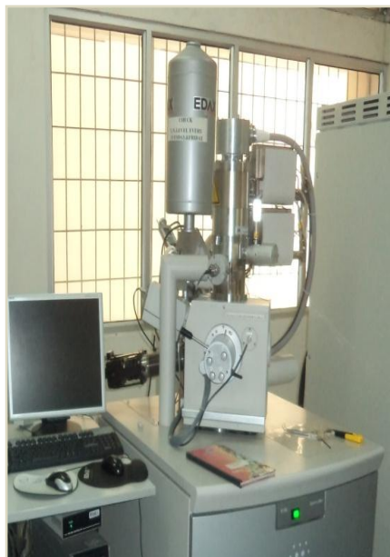
Fig. 3.5 A photograph of FEI Quanta 200F scanning electron microscope.
