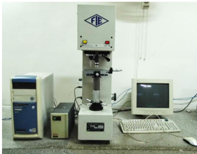
Figure 3.3: Computerized Vickers Hardness Tester ( FIE-Model:VM 50 PC)
