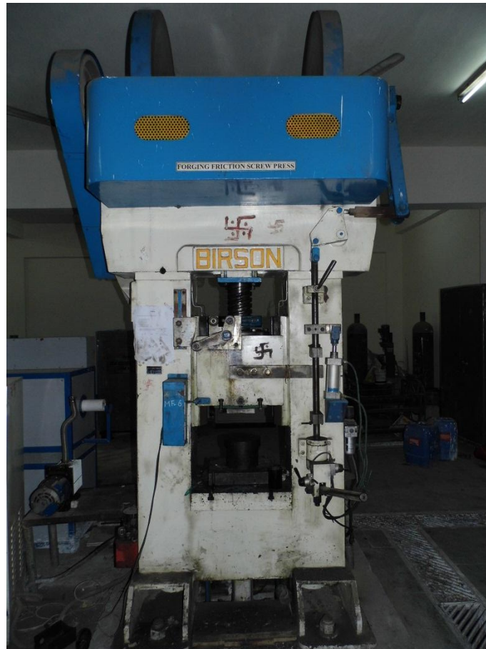
Figure 3.2: Friction screw forging press used for Multi axial forging
