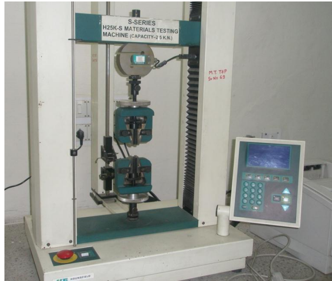
Figure 3.4: S-Series, H25K-S tensile testing machine.
