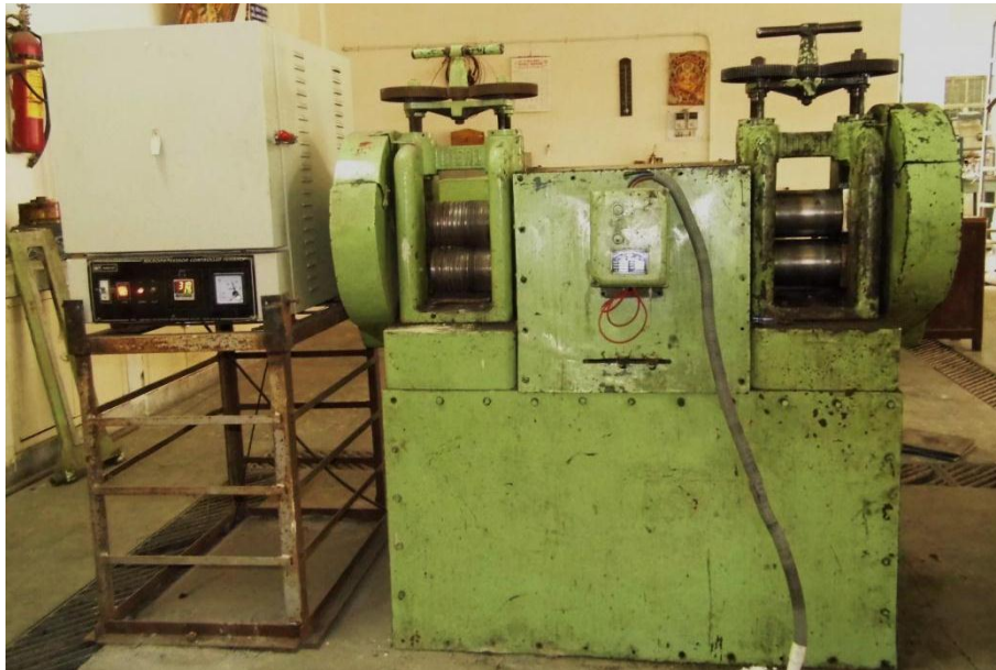
Figure 3.1: Two high rolling mill used for cryorolling
