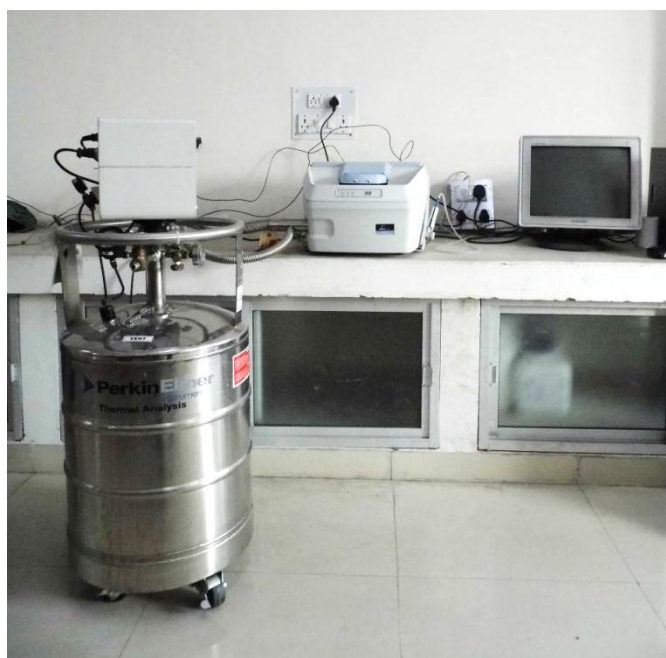
Figure 3.7: Perkin Elmer's DSC 8000 series machine.
