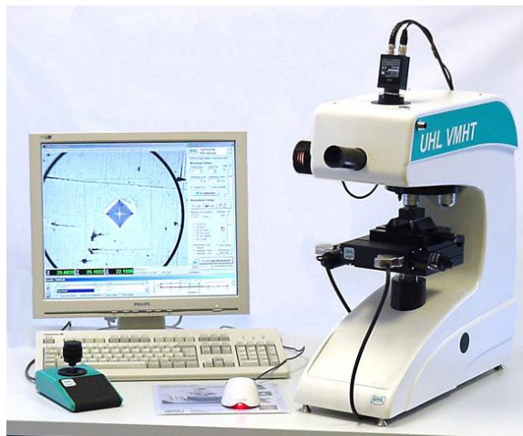
Figure 2.23 Photograph of Microindenter (UHL VMHT)
