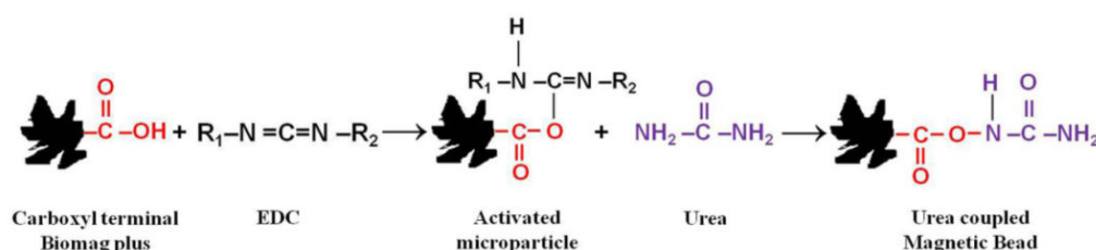
Fig 4.1A Urea immobilization: EDC assisted coupling of urea to carboxylic magnetic beads.
