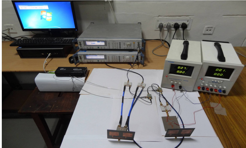
Figure 5.9: Measurement setup for NIVSD using indigenous and laboratory equipment [125].
