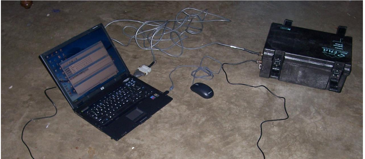
Figure 2.8 Retrieval of data recorded in the strong motion accelerograph through a cable by using the laptop.
