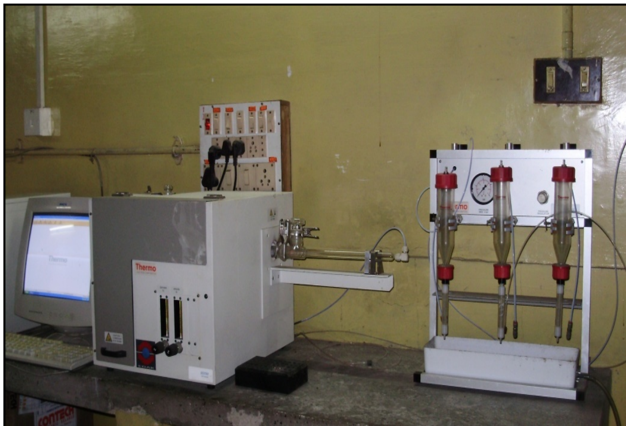
Figure 2.5: AOX analyzer (Dextar AOX analyzer, Thermo Electron Corporation)
