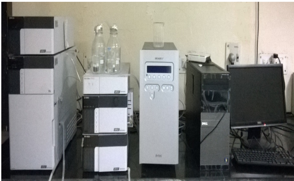
Figure 2.3: High Performance Liquid Chromatography (Shimadzu LC-20 AD)
