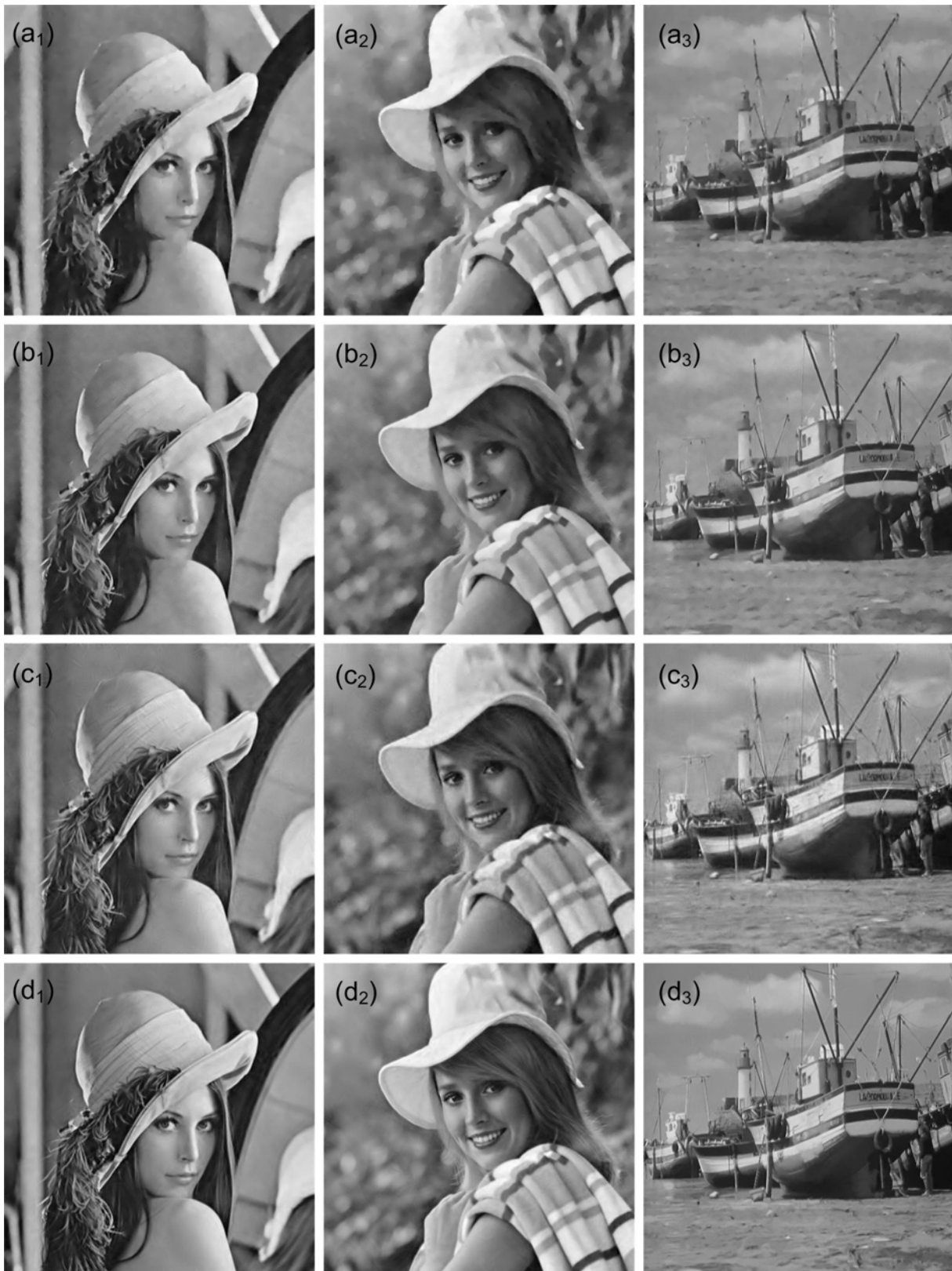
Figure 5.16 Visual denoising performance obtained by the (a) ADF (b) NLMF (c) CSST (d) Proposed NSST-NLNADF. Here 1, 2 and 3 refer to Lena, girl and boat images, respectively
