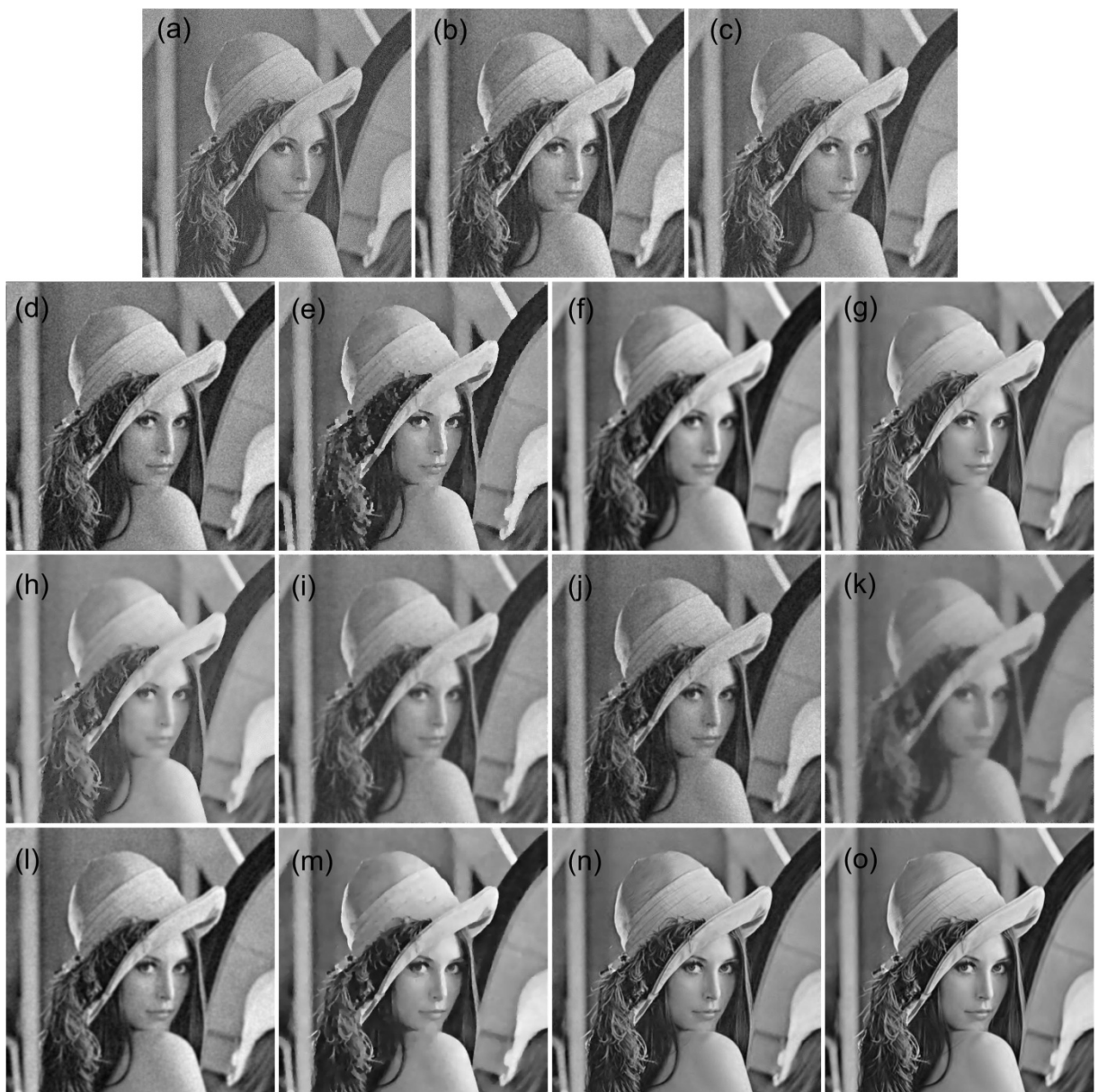
Figure 5.23 Comparative visual performance of (a) Lena image corrupted by Gaussian noise and processed by the (b) AWMF (c) WF (d) Kuan (e) LHMAF (f) MHOPNF (g) FOPDEF (h) SRAD (i) NCDF (j) INCDF (k) SBF (l) SRBF (m) TVF (n) NSST-NADF (o) NSST-NLNADF
