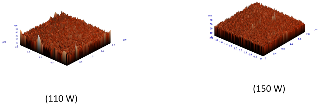
Figure 5.7 AFM micrographs of film deposited at different sputtering power of titanium.
