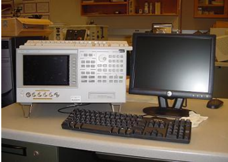
Figure 2.16 Impedance analyzer used for measurement of capacitance of thin film
