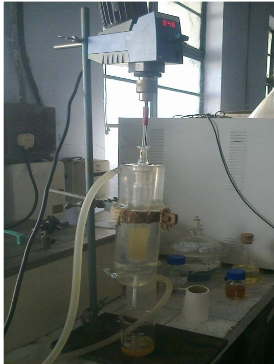
Figure 4.1. Actual photograph of glass mixer-settler for single stage equilibrium extraction.
