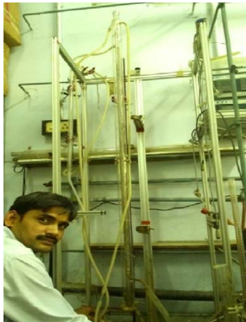
Figure 4.2. Picture of actual experimental set up for continuous counter current extraction.
