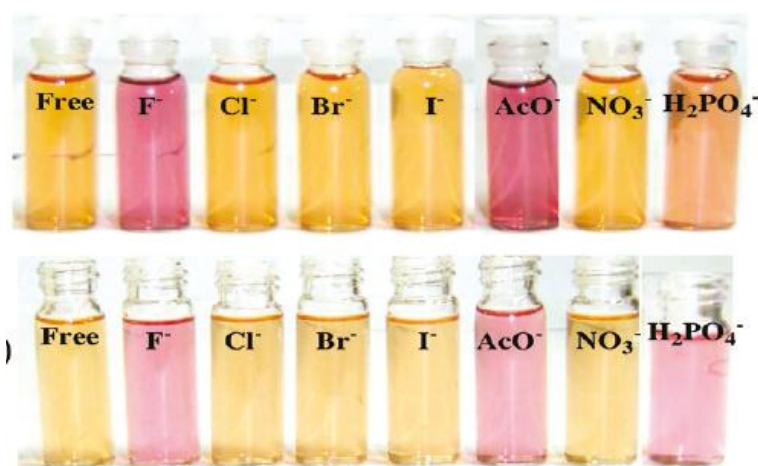
Fig. 3.31 Color changes in metalloreceptor before and after the addition of anions
