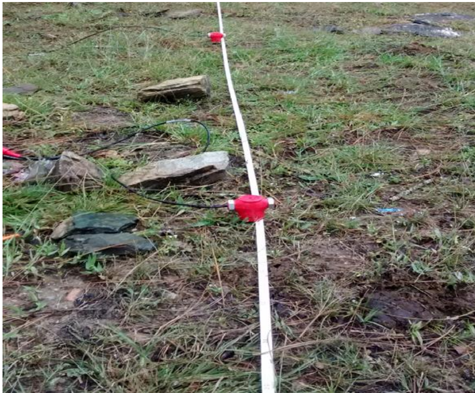
Figure 4: Set up geometry of Geophones array. East-West Profile.
