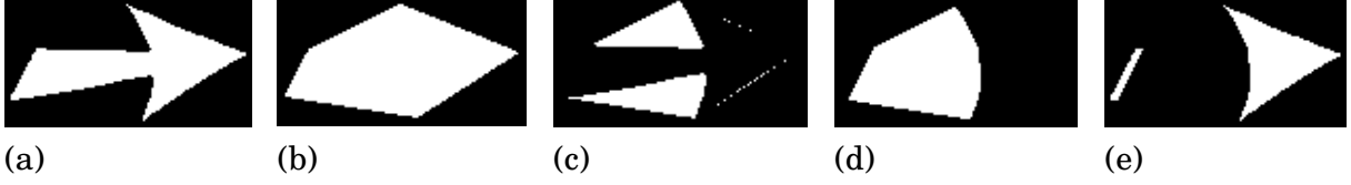
Figure 3.4: Arrowhead candidate cropping: (a) an arrow, (b) convex hull, (c) convexity defect, (d) a complete convexity defect region, and (e) arrowhead candidates.
