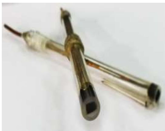
Fig. 1.7: An edge plane pyrolytic graphite electrode used for voltammetric determinations.
