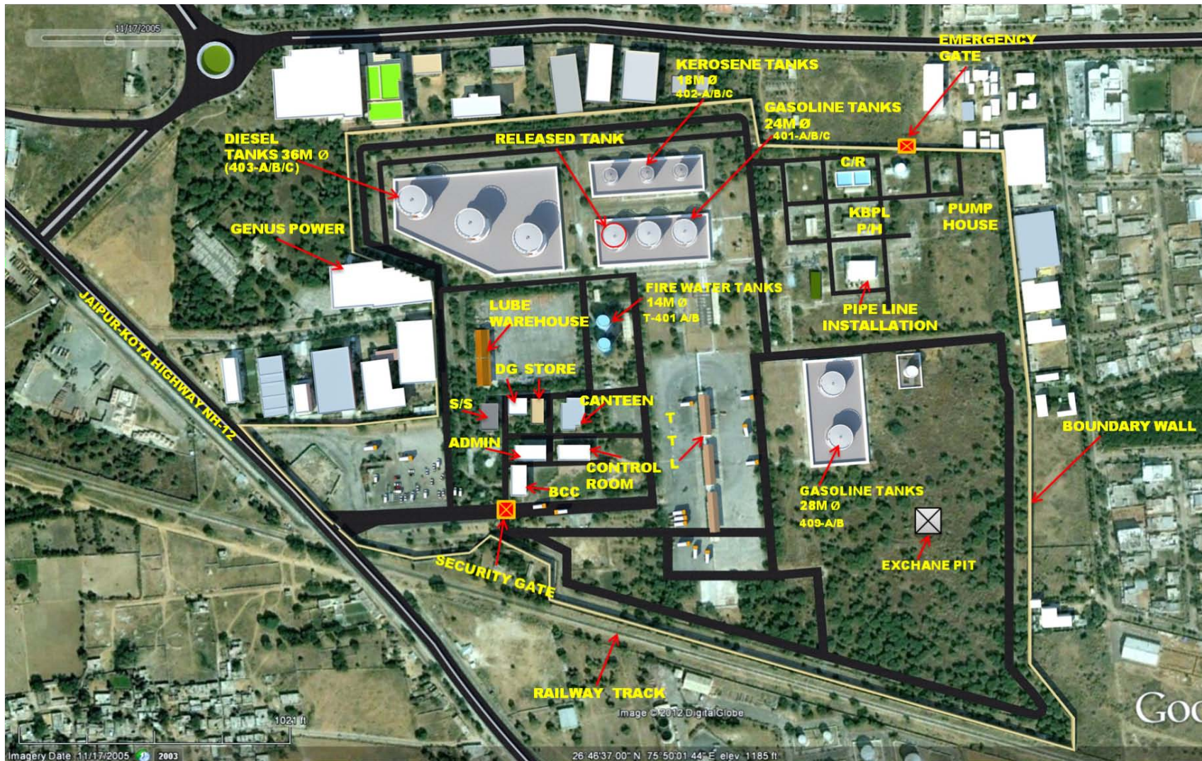
Fig. 3.3 Pre-accident arial view of IOCL Jaipur terminal tank storage site and the immediate neighbourhood
