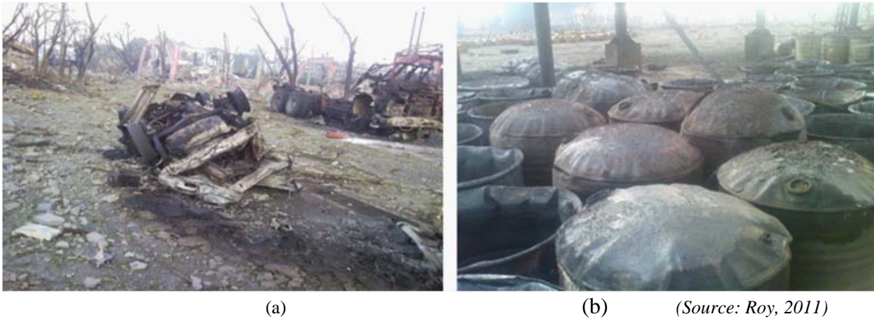
Fig. 4.7 (a) Damaged Vehicles and (b) lube oil drums due to extensive over pressure of vapour cloud explosion
