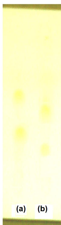
Fig. 4.4: Chromatograms in line (a) and (b) are showing resolution of diastereomers of ( RS )-Flx prepared with CDR 4 and 5, respectively. Chromatographic conditions: as mentioned in the legend of Table 4.2.
