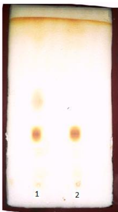
Fig. 3.14: Photograph of an actual chromatogram showing resolution of (RS) -AtI using approach (A). From left to right: Line 1, (R:S) , 1:99, lower spot for (S) -isomer and upper spot for (R) -isomer; line 2, is of (S) -isomer. Chromatographic conditions are the same as in Fig. 3.10.
