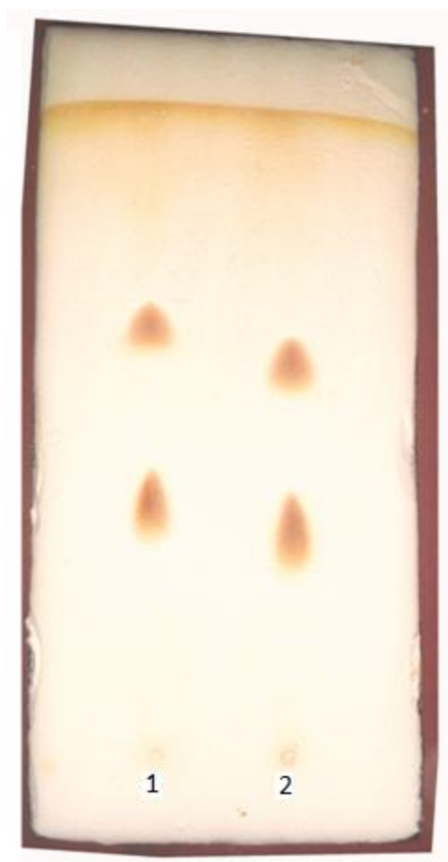
Fig. 3.11: Photograph of an actual chromatogram showing resolution of ( RS )-Orc and ( RS )-Bel on the plates impregnated with L-Glu (approach (A)); from left to right: Line 1 and 2, respectively, for ( RS )-Orc and ( RS )-Bel, lower spot is of ( S )-isomer, and the upper spot is of ( R )-isomer resolved from the racemic mixture. Chromatographic conditions are the same as in Fig. 3.10.
