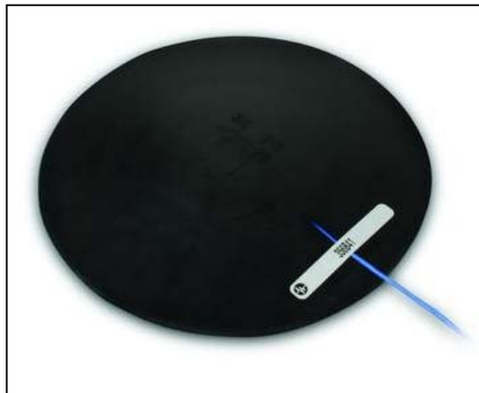
Fig. 3.4 PCB Triaxial accelerometer mounted on floor
