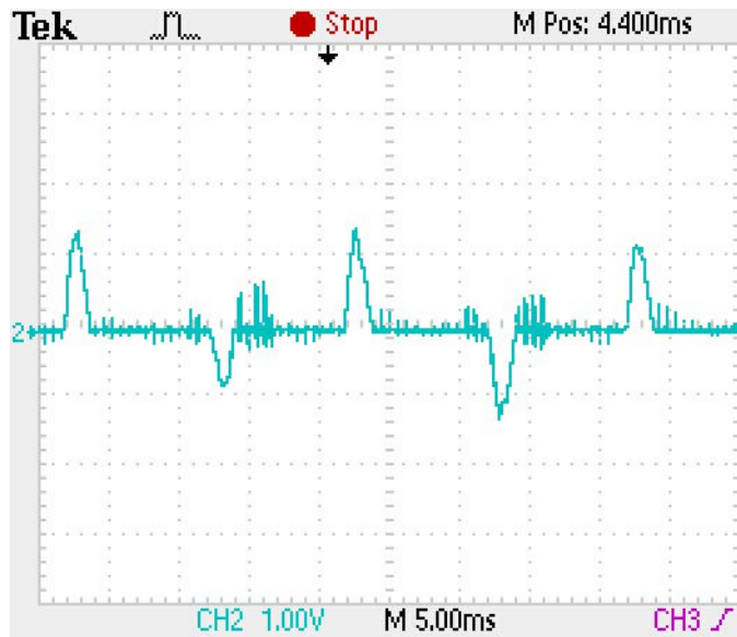
(b) Experimental ( Input AC current: 1 amp per division, Time scale: 5ms per division )
