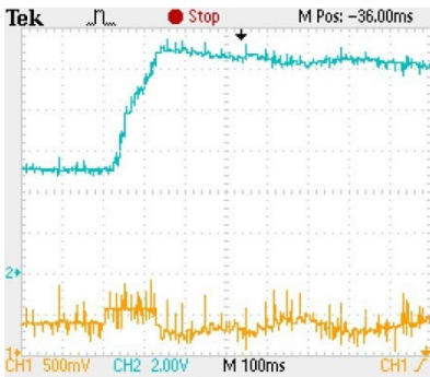
(d) Experimental: 500rpm to 1000 rpm, settling time T_{sett} = 0.9 sec ,(CH1: duty cycle 0.5 per division, CH2: speed 200 rpm per division)
