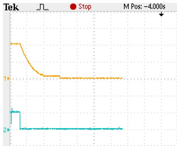
(b) Experimental: retardation time 1.8 sec (CH1: speed 500rpm per division, CH2: PWM duty cycle 0.25 per division)
