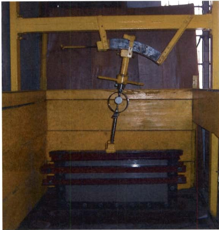
Figure 3.5 Test set-up arrangement for model tests (Plane strain condition)
