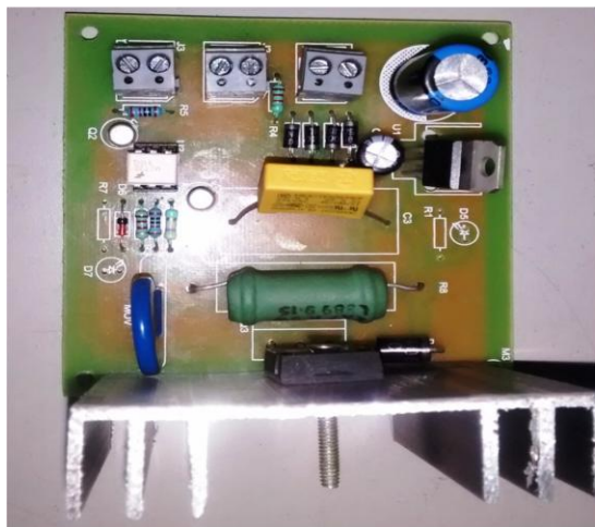
Figure 9.9 : Driver circuit and its output pulses
