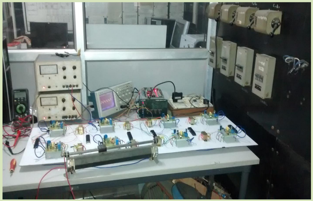
Figure 9.8: Hardware setup of 5-level H bridge inverter (open loop)
