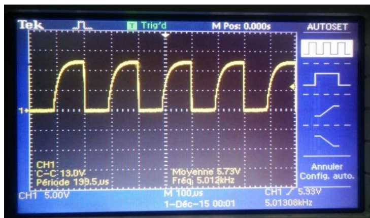
Figure 6.4 Firing Pulses of Driving Circuit Using MCT2E
