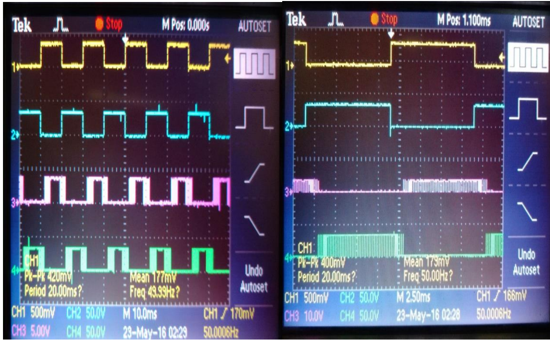
Figure 6.11 Switching States Of Heric Inverter
