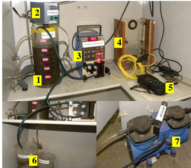
Figure 5.3.2. Actual photograph of experiment setup. (1) Reactor, (2) Agitator, (3) Peristaltic Pump, (4) Rotameter, (5) pH/DO meter, (6) Discharge collection beaker, (7) Compressor
