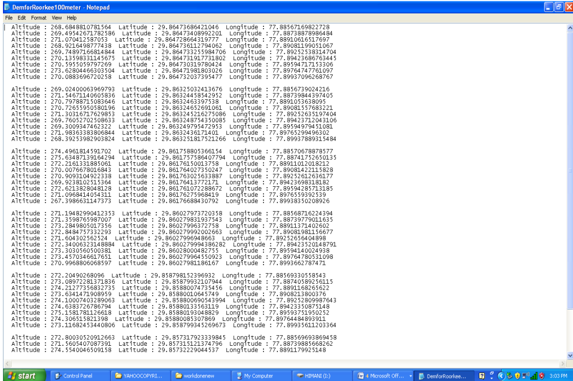
Figure 6.40: DEM file showing Altitude, Latitude and Longitude for Roorkee area at a grid interval of 100 Pixel
