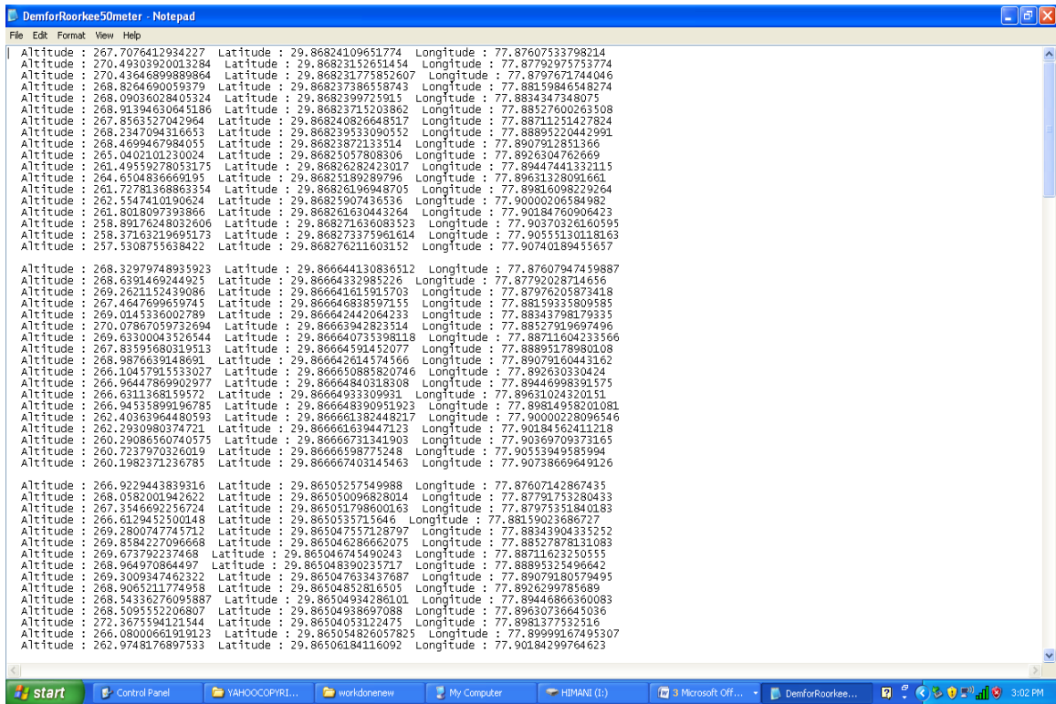
Figure 6.38: DEM file showing Altitude, Latitude and Longitude values for the Roorkee area at a grid interval of 50 Pixel
