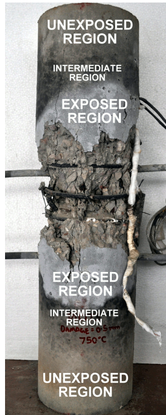
Fig. 3.17: Thermal Gradient evident from color change
