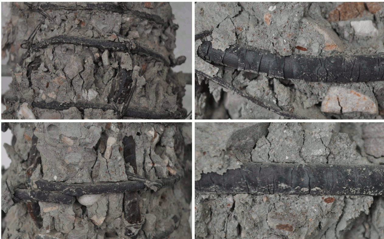
Fig. 3.28: Confinement failure at 750 °C
