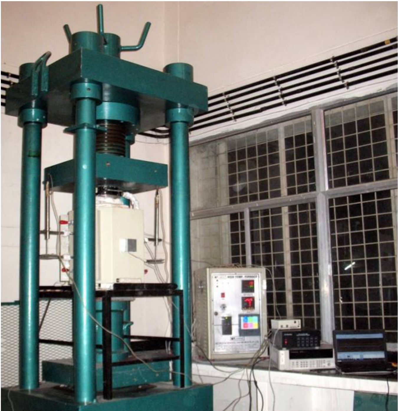
Fig. 3.8: Actual test setup with elevated temperature testing in progress
