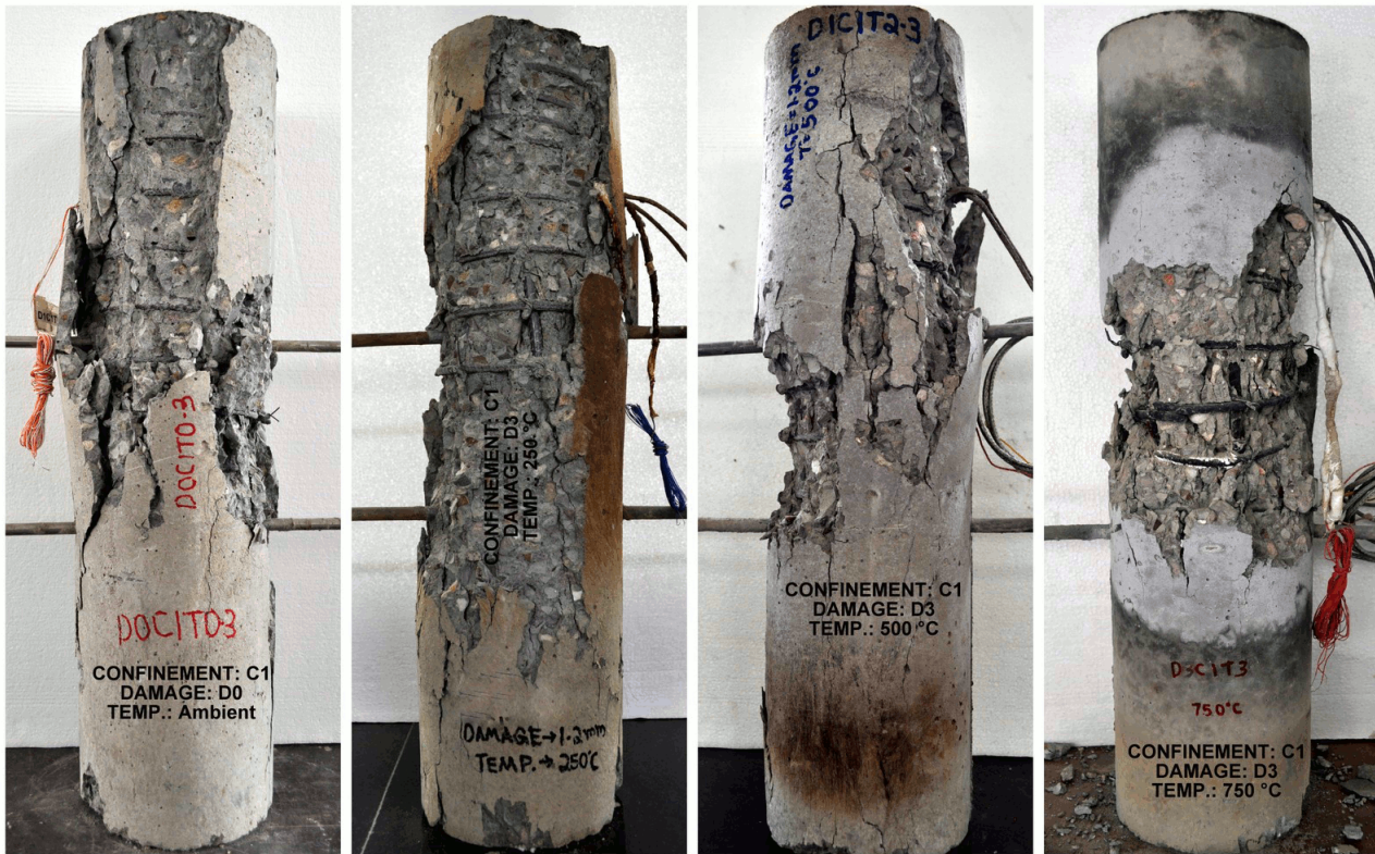
Fig. 3.24: Failure of specimens with confinement C1 under damage category D3
