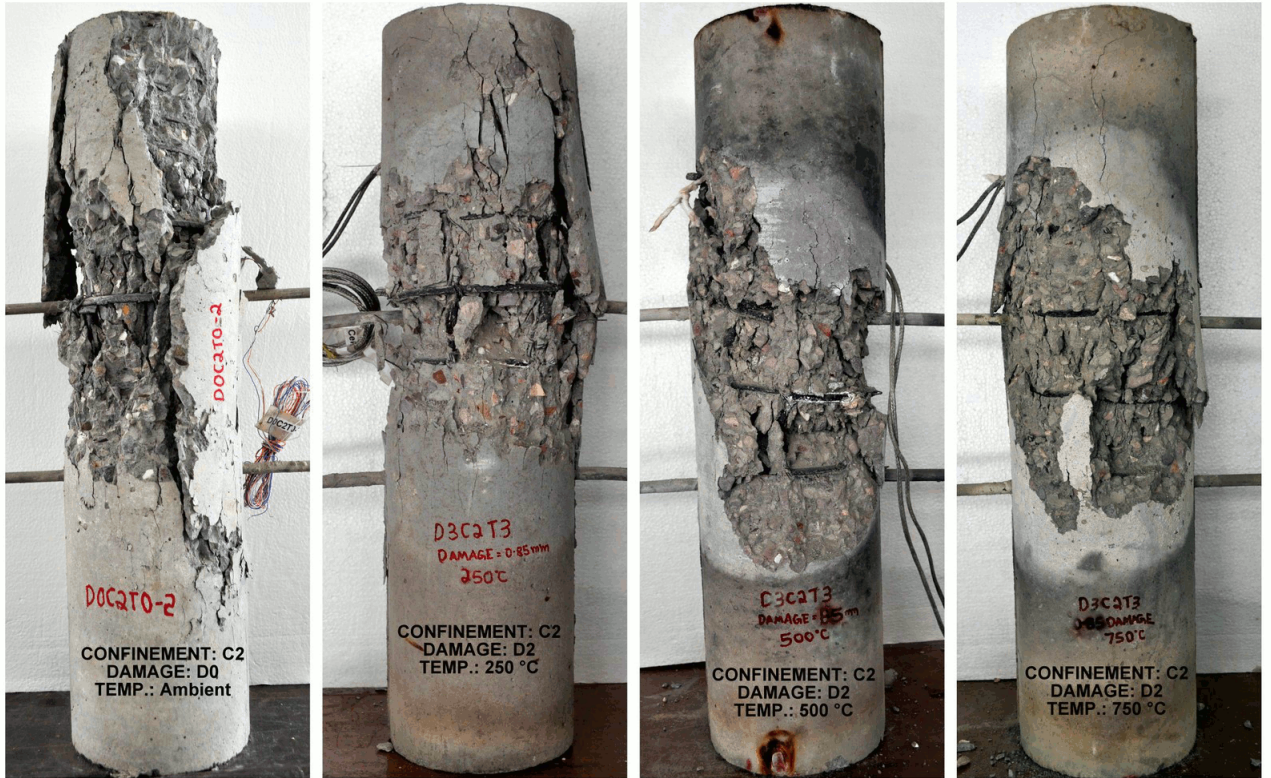
Fig. 3.26: Failure of specimens with confinement C2 under damage category D2
