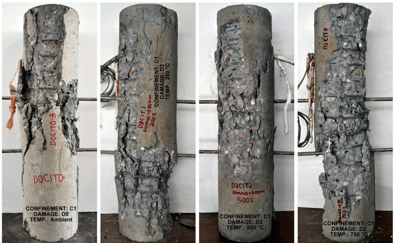
Fig. 3.23: Failure of specimens with confinement C1 under damage category D2
