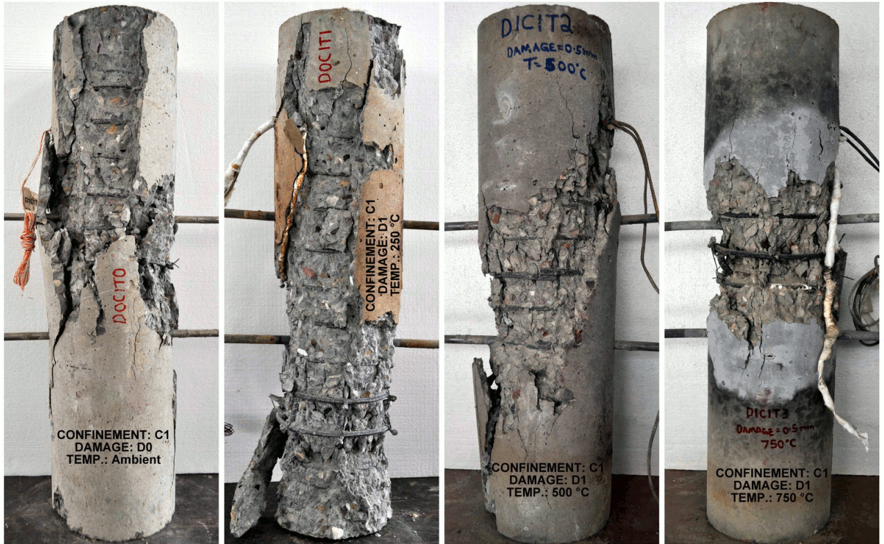
Fig. 3.22: Failure of specimens with confinement C1 under damage category D1
