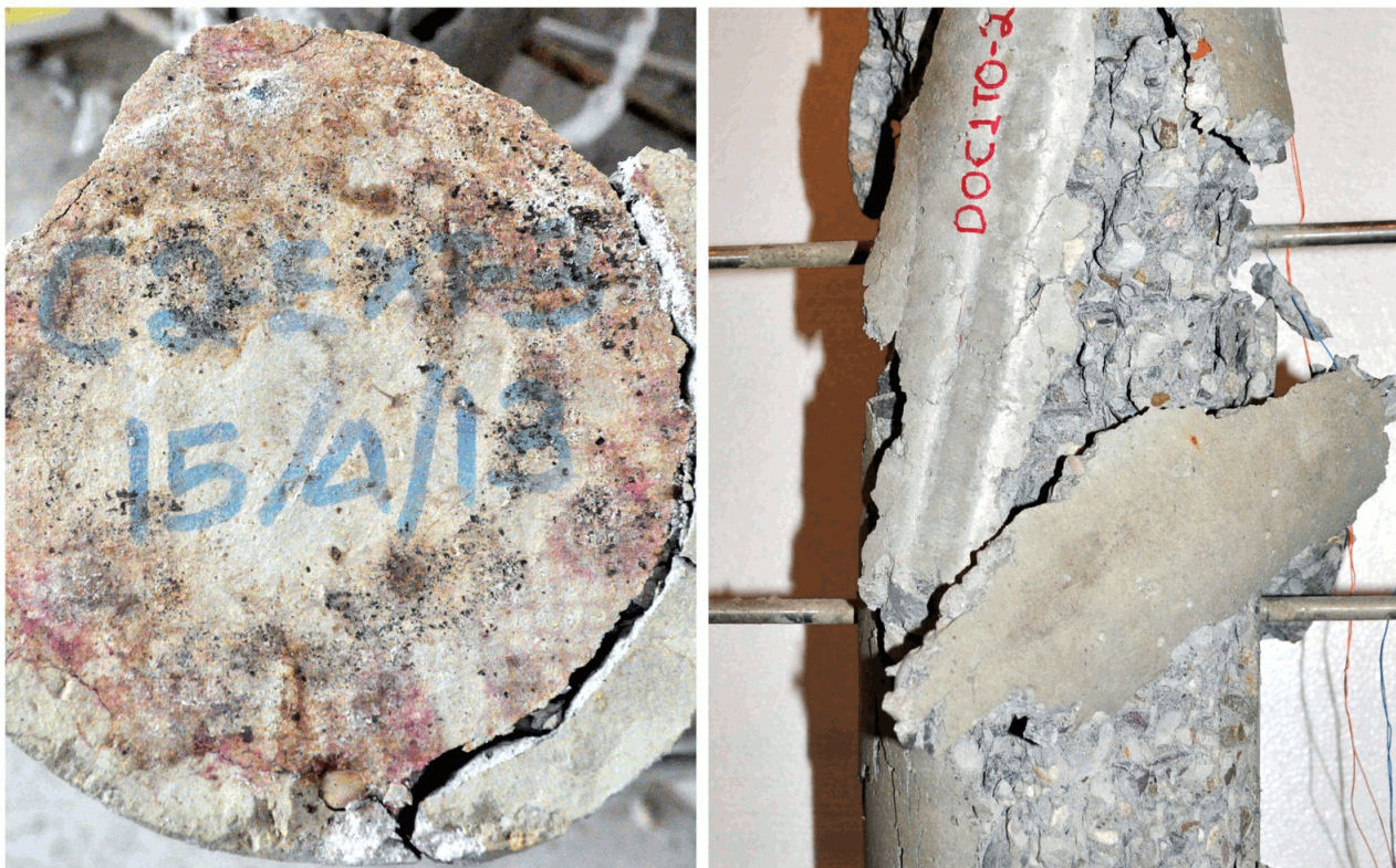
Fig. 3.21: Loss of cover concrete
