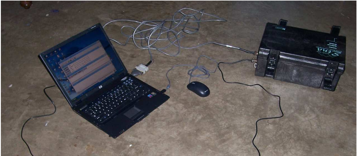
Figure 5.8: Retrieval of data recorded in the accelerograph through a cable by using the laptop.
