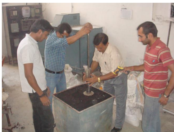
(e) Compaction of DBM by dynamic loading
