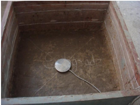
(a) Load cell placed at top of subgrade
