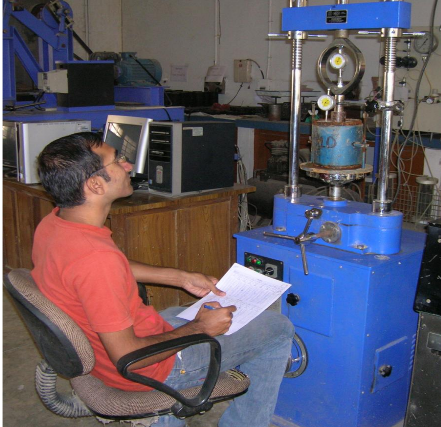
Figure 3.7 Laboratory Setup for Determination of CBR
