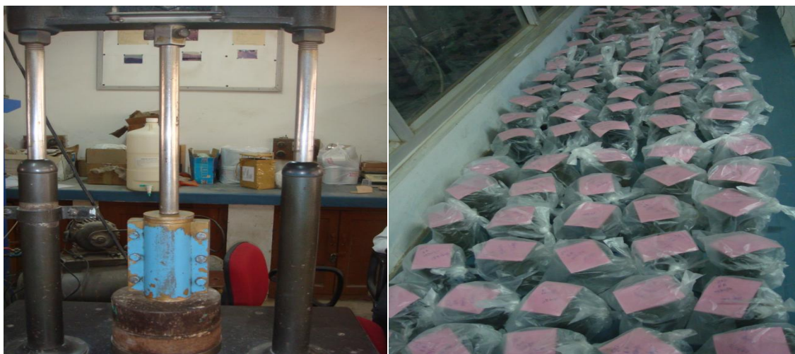
(b) Compacted Specimens Kept in Polyethylene Bag
