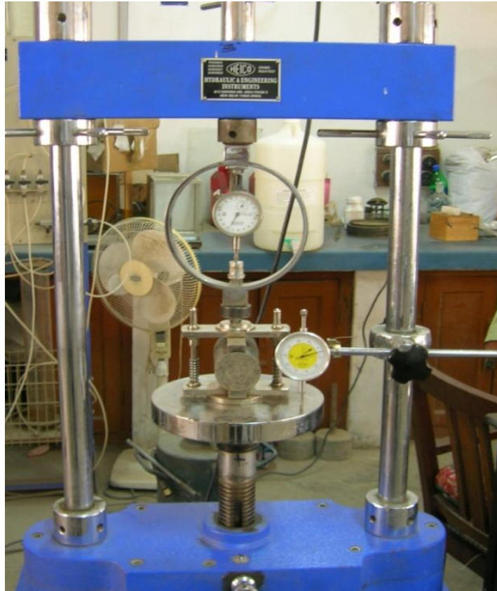
Figure 3.13 Test Setup for Split Tensile Strength Test
