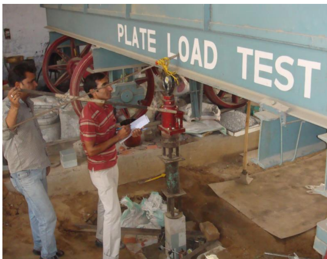
Figure 3.16 Test Setup for Plate Load Test
