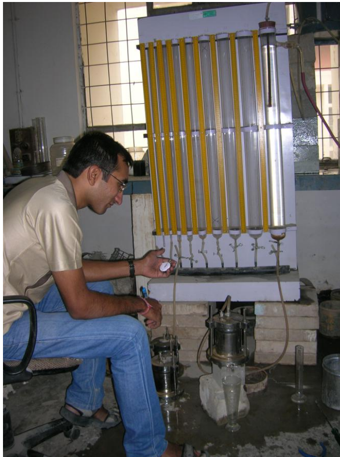
Figure 3.11 Laboratory Setup for Determination of Permeability
