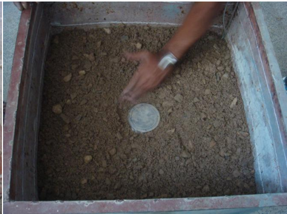
(b) Load cell at interface of sub base and WMM
