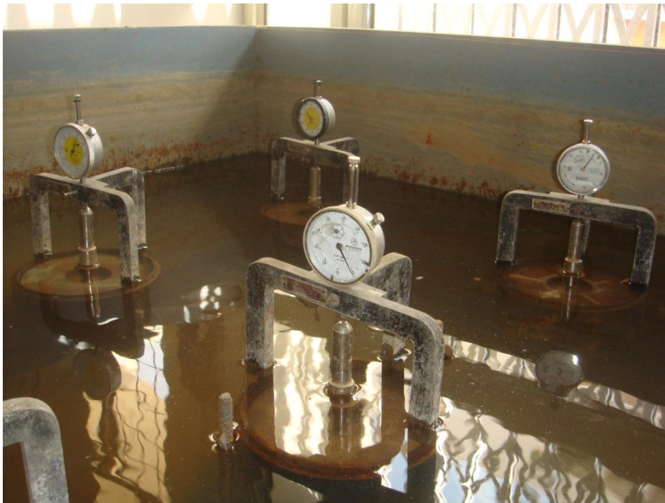
Figure 3.6 Laboratory Setup for Determination of Expansion Ratio
