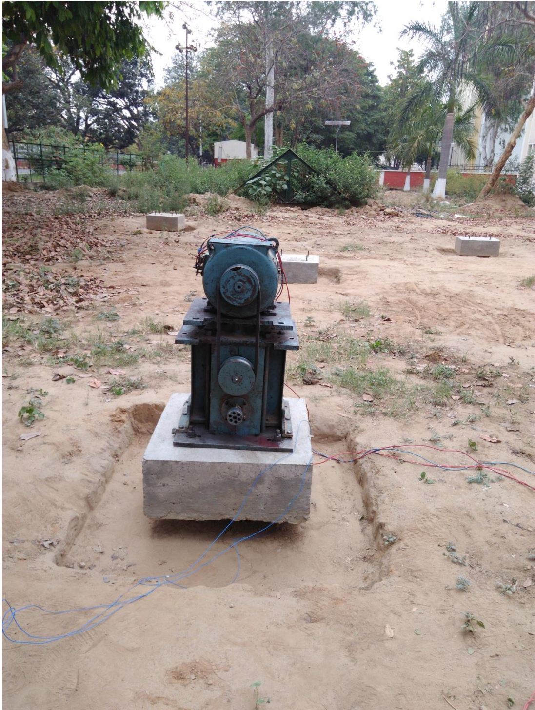
Figure 4-1 Lateral Forced Vibration Setup
