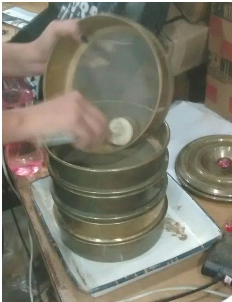
Figure3-2 Performing Grain size analysis
