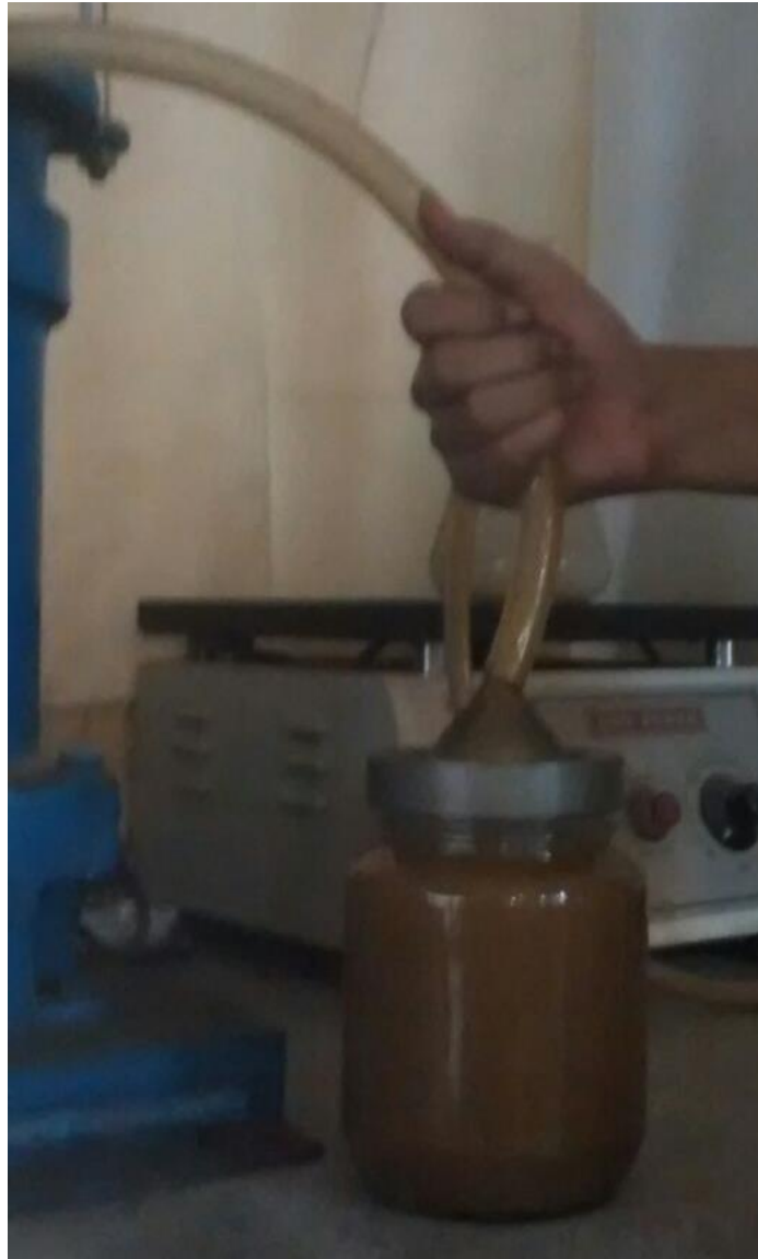
Figure 3-7 Performing pycnometer test
