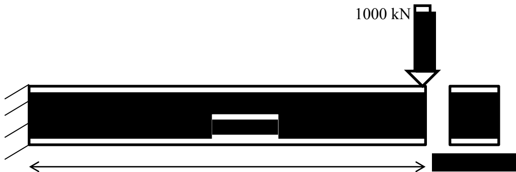
Fig.4.1: Elevation of Cantilever Beam Model
