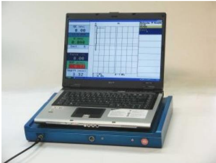
Fig. 3.3 Data acquisition system used in CPTu test
