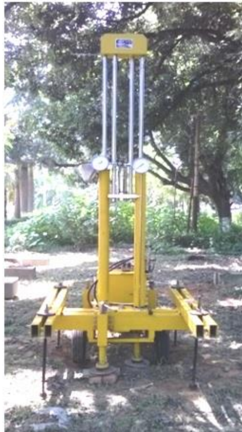
3.1(b) Set up of CPT in field
