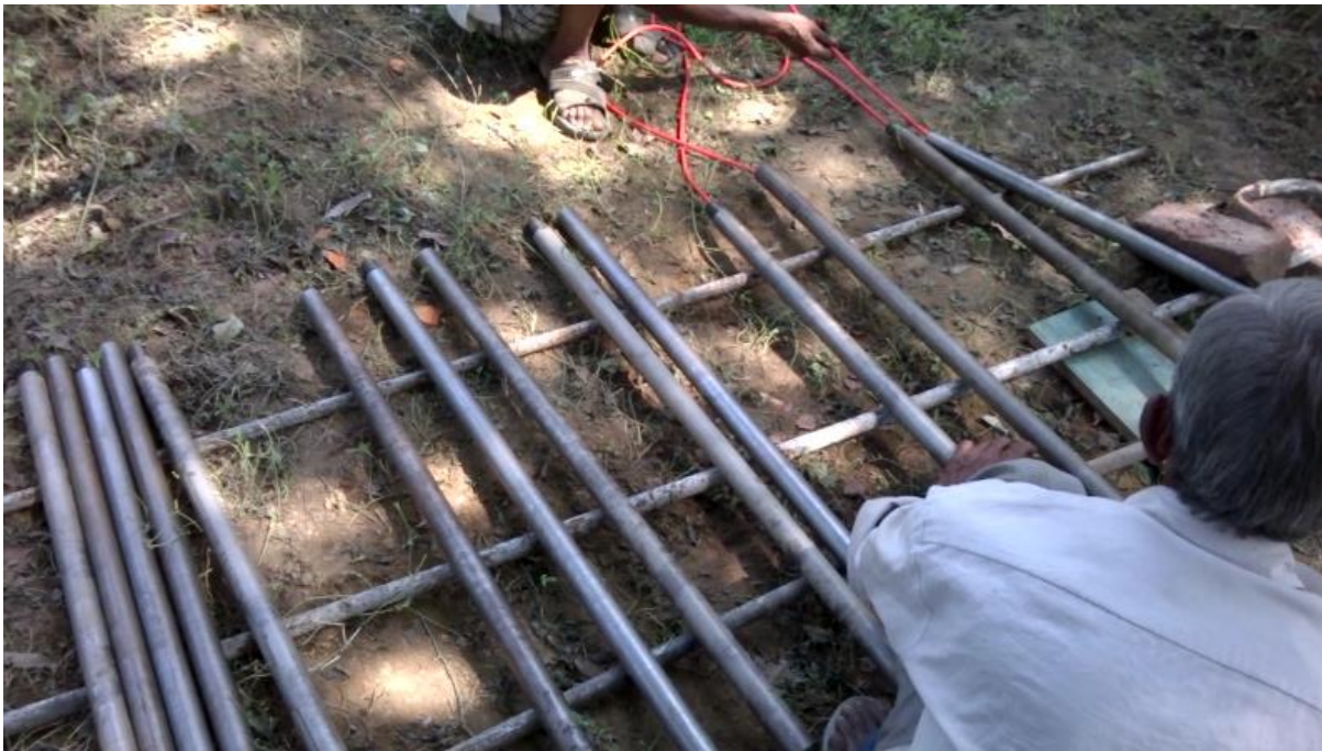
Fig. 3.2(b) sounding rods arrangement for CPTu test
