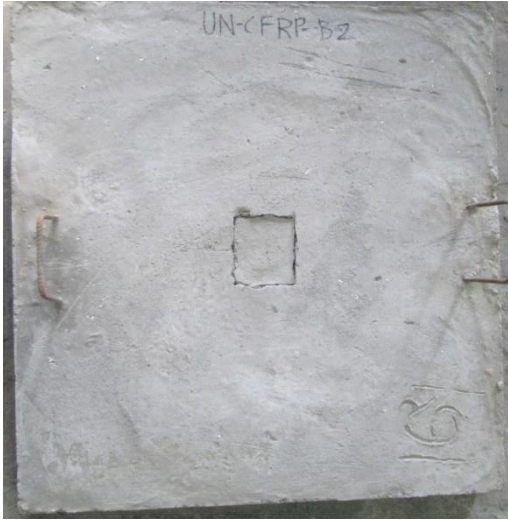
Figure 5.17 (a) Punching on top face of USC-70
