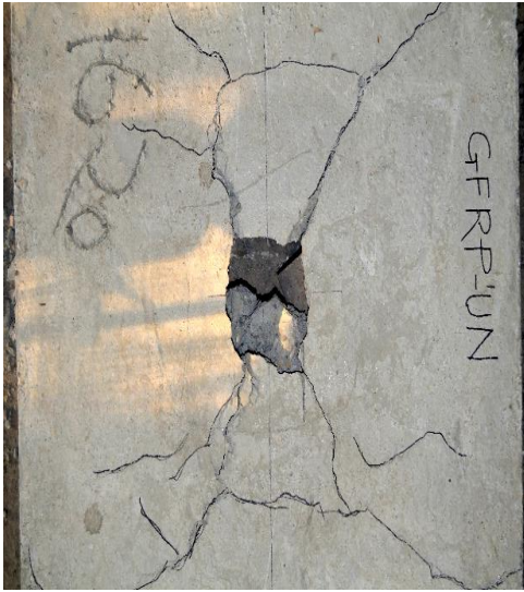
Figure 5.14 (a) Cracks on top face of USG-100
