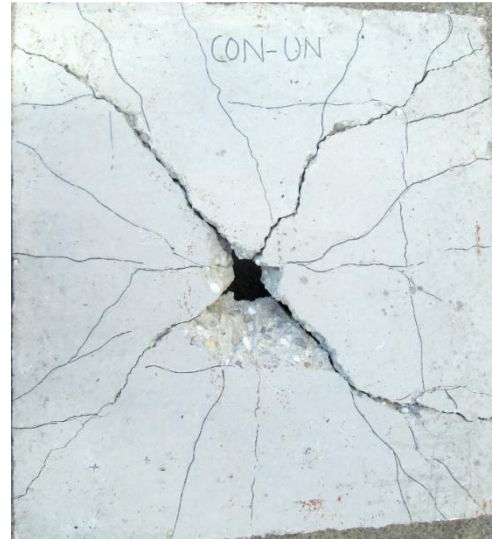
(b) Cracks on bottom face of UC
