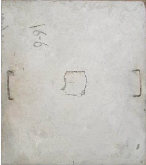
Figure 5.10 (a) Punching on top RSC-100
