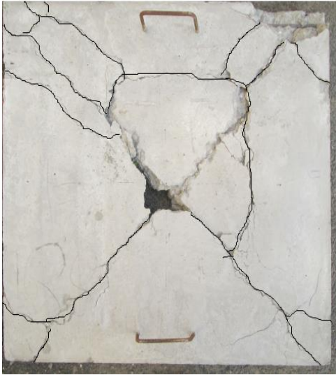
Figure 5.13 (a) Cracks on top face of UC
