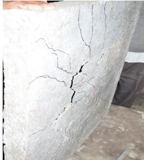
(b) Central punching failure region.
