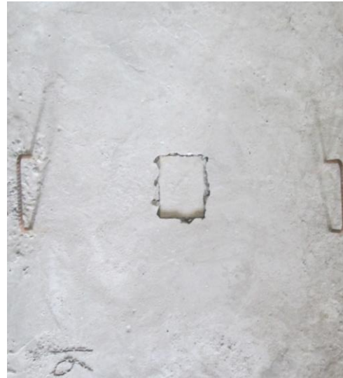
(b) Punching on top of RSG-100
