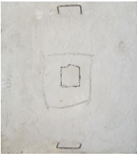
Figure 5.15 (a) Punching on top face of USC-100
