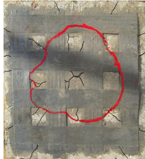
(b) Cracks on bottom face of RSC-100
