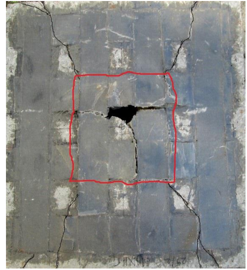
(b) Cracks on bottom face of USG-100
