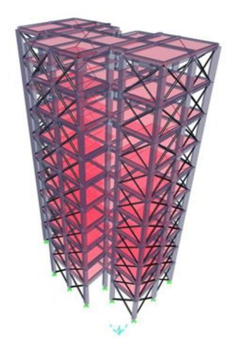
Fig.4-2-Model of building with steel bracing addition
