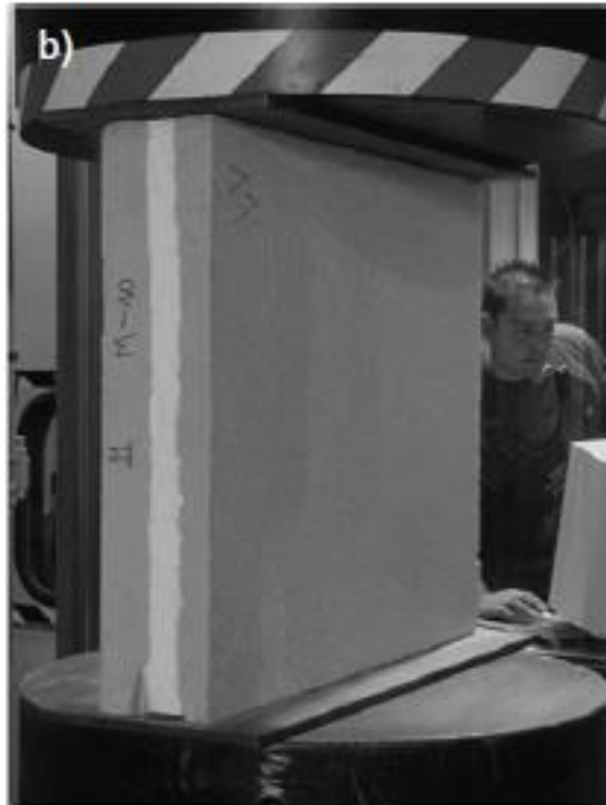
Figure 1.6: Compression test setup (Source: Carbonari et al. (2012))
