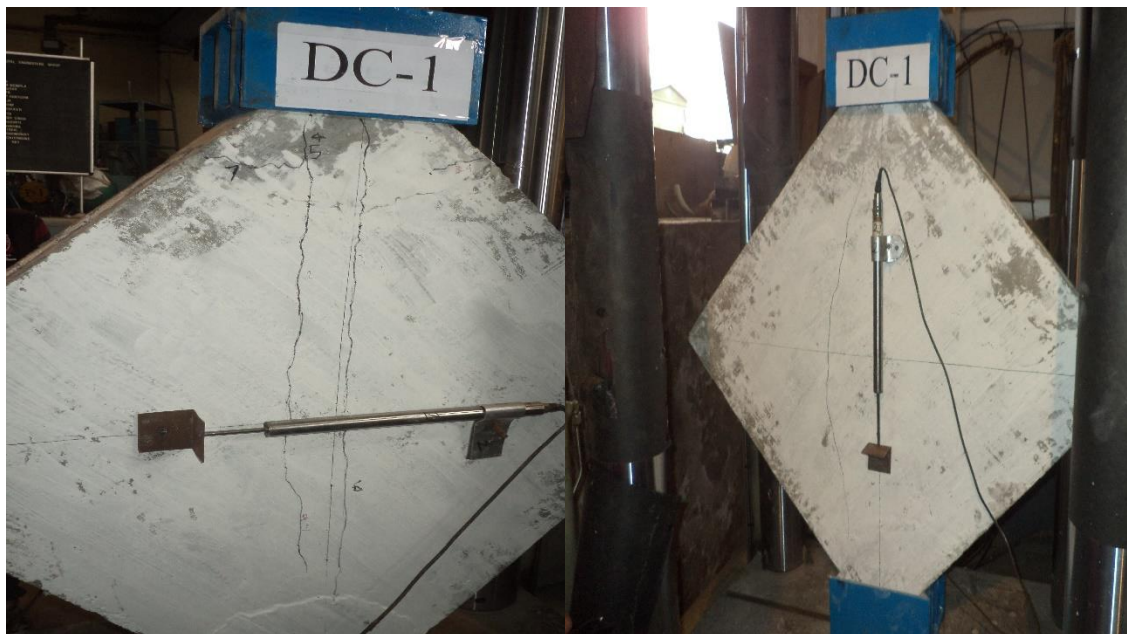
Figure 2.2: Crack pattern observed in diagonal compression test
