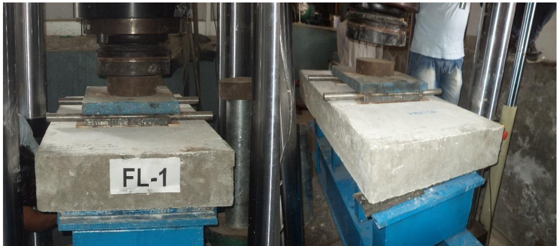
Figure 3.1: Test setup and loading condition of flexural test
