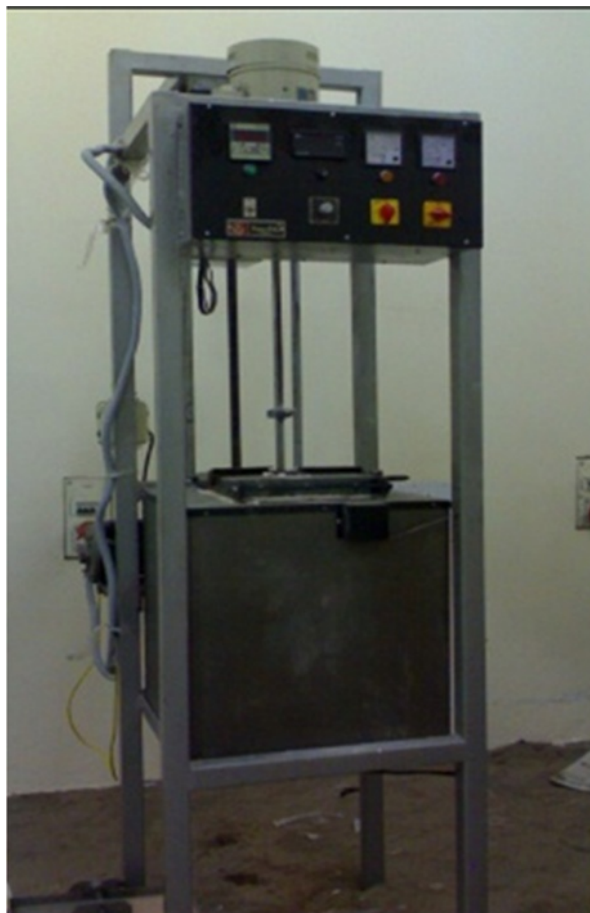
Figure 3.1. Stir casting set-up [12]
