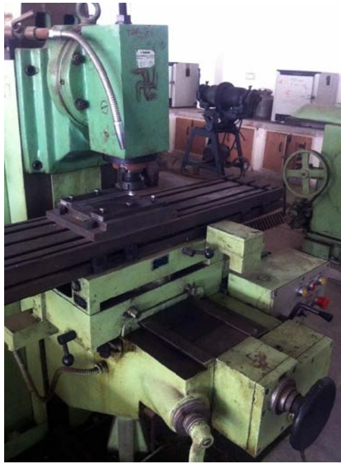
Figure 3.3. Vertical milling machine set-up for conducting FSP[14]
