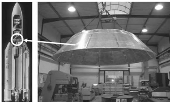
Fig. 17. Aluminum foam sandwiched is being used in Ariane 65 rocket
