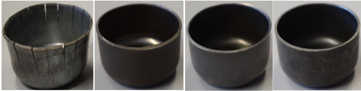
a) Cracks initiate from cup rim b) No crack appeared from last five months c) No crack appeared from last five months d) No crack appeared from last five months
