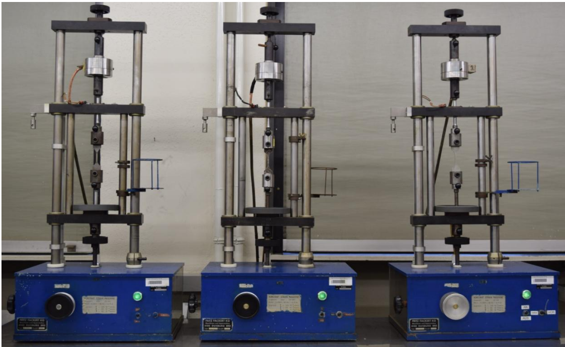
Figure 4.4: The constant extension machine with maximum load of 30 kN for performing slow strain rate test.
