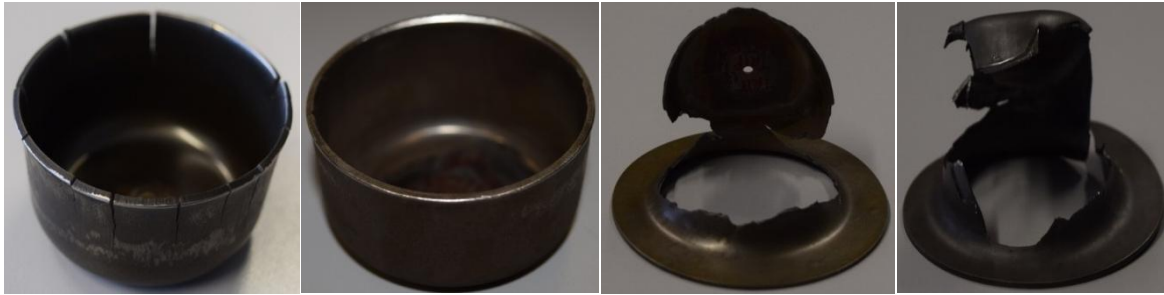
a) Cracks initiate from cup rim b) No crack appeared from last four months c) Not able to form a cup because material loses its formability due to high amount of hydrogen d) Not able to form a cup because material loses its formability due to high amount of hydrogen
