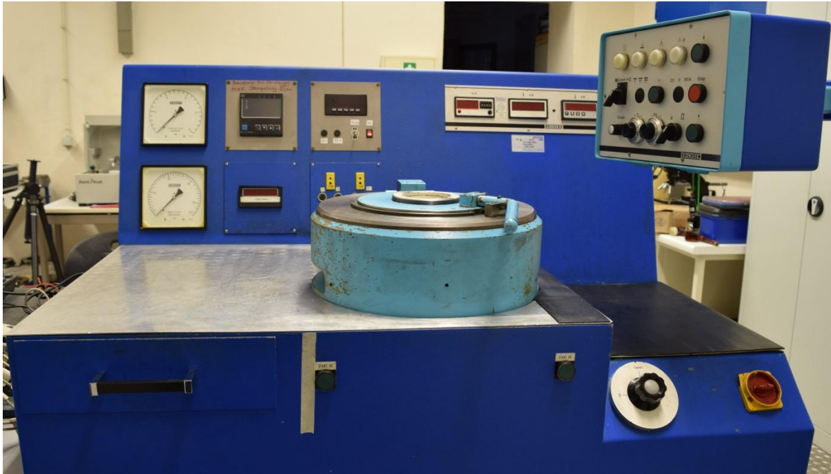
Figure 4.5: ERICHSEN 142/40 sheet testing machine for deep drawing test.
