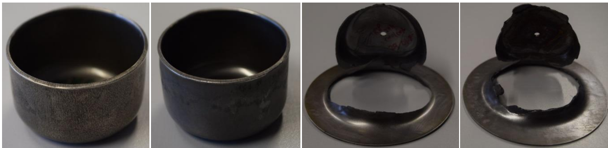
a) No crack appeared from last two months b) No crack appeared from last two months c) Not able to form a cup because material loses its formability due to high amount of hydrogen d) Not able to form a cup because material loses its formability due to high amount of hydrogen
