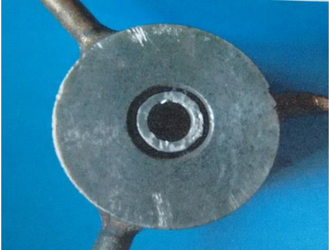
Fig. 4.2 Picture of closed type gas atomizer used in spray forming
