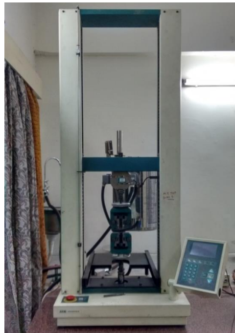
Fig. 4.12 Universal testing machine (Tinius Olsen, Model:H25KS)
