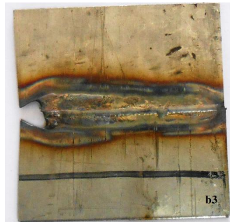
Fig.20 Weld bead shape of sample at face and root, welded at 2mm/s with high heat input
