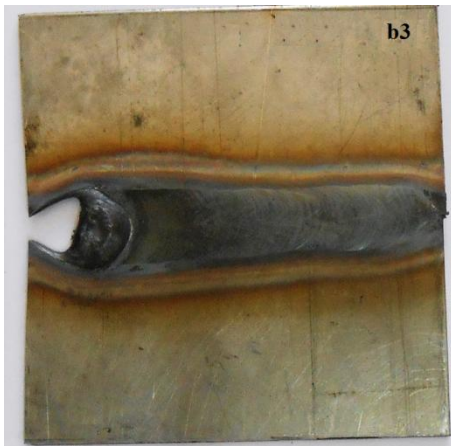
Fig.20 Weld bead shape of sample at face and root, welded at 2mm/s with high heat input
