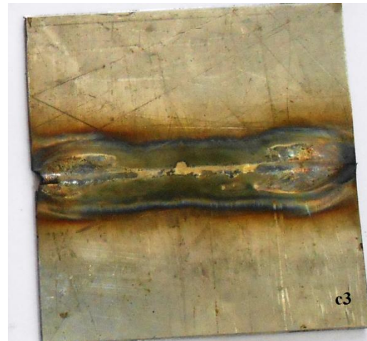
Fig.23 Weld bead shape of sample at face and root, welded at 3mm/s with high heat input
