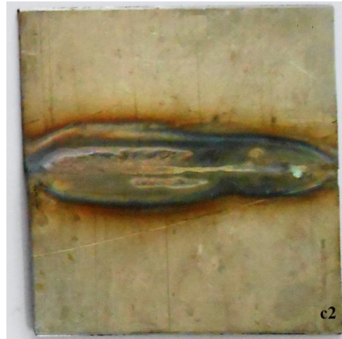
Fig.22 Weld bead shape of sample at face and root, welded at 3mm/s with medium heat input
