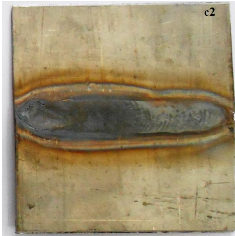
Fig.22 Weld bead shape of sample at face and root, welded at 3mm/s with medium heat input
