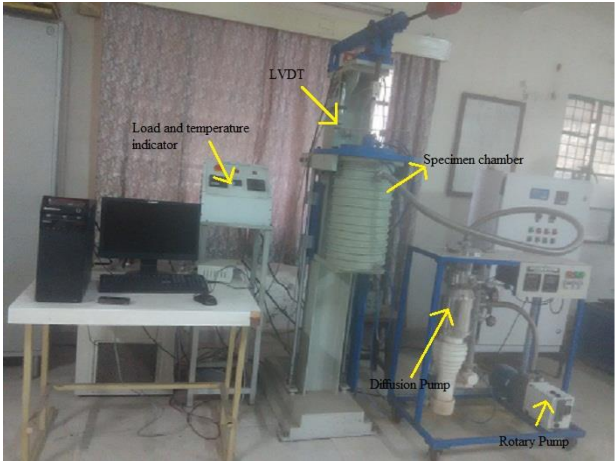
Fig.5.9- Indentation creep testing machine set up
