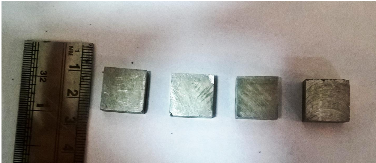
Fig. 5.8- Sectioned samples for creep testing
