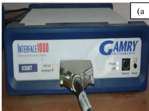
Figure 13 (a) Gamry interface 1000 (b) Electrochemical cell with three electrodes
