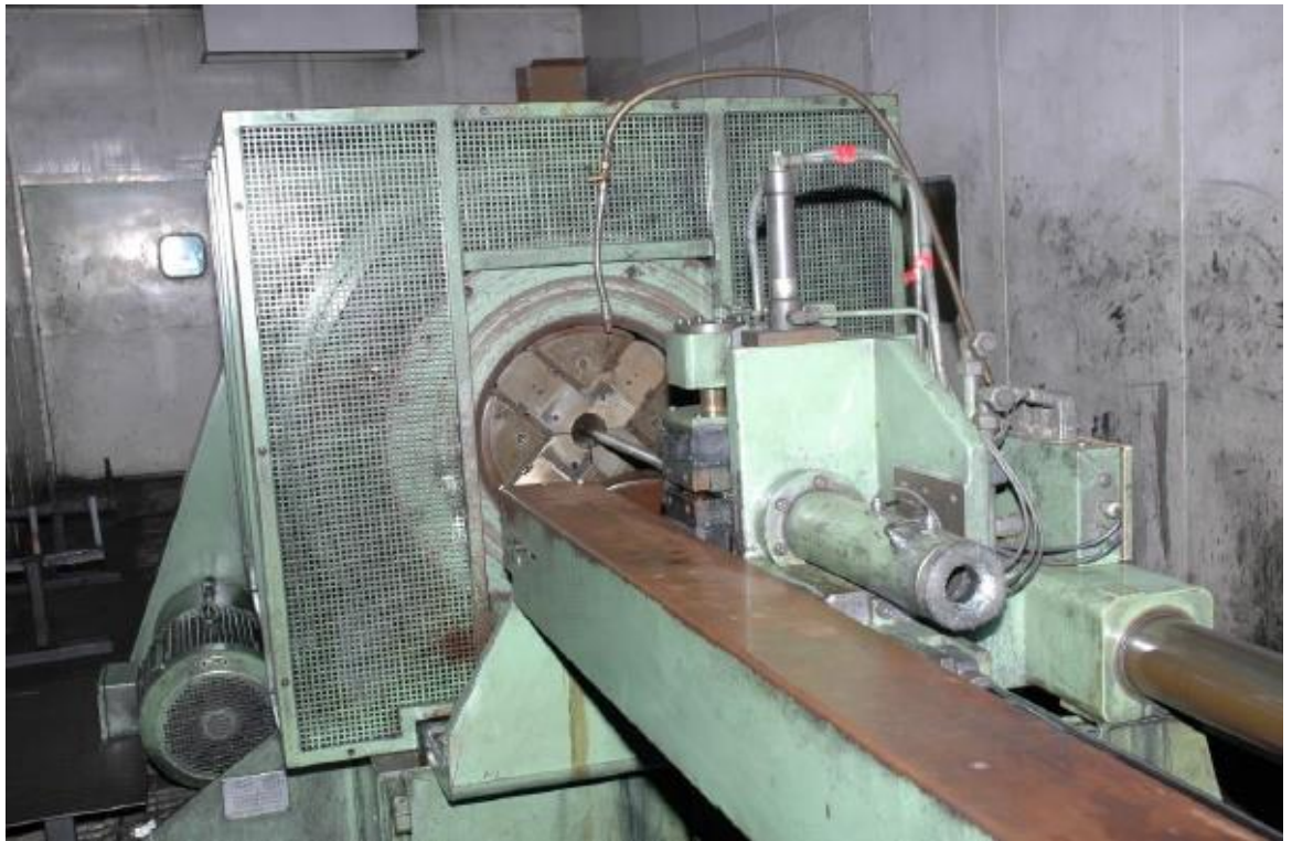
Figure 6 Rotary swaging machine at nuclear fuel complex, Hyderabad.
