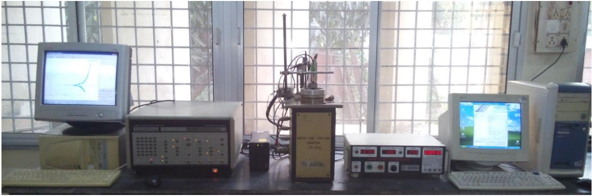
Fig.12. Experimental set-up to evaluate the tribocorrosion behaviour
