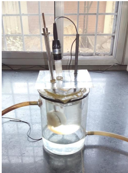
Fig.10. Glass cell with inlet and outlet for hot water circulation showing electrode positions
