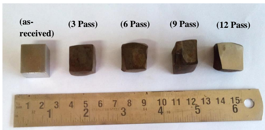
Fig.15. Warm multi-axially forged 316L SS samples of as-received, 3 pass, 6 pass, 9 pass, and 12 pass conditions
