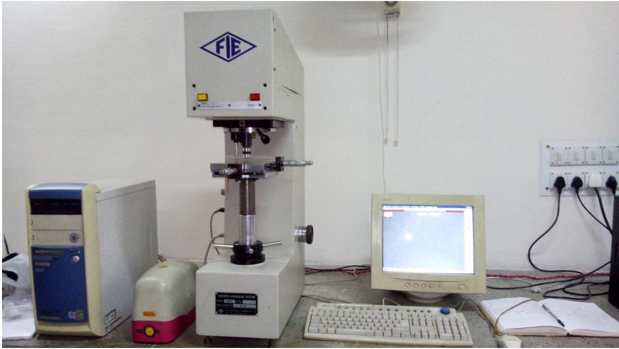
Fig.8. FIE-VM50 PC Vickers hardness testing machine
