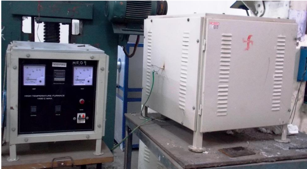
Fig.4. Muffle furnace for heating the samples prior to MAF
