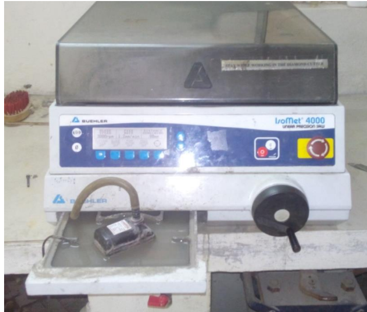
Fig.5. Buehler Isomet 4000 saw used to cut the samples with required precision
