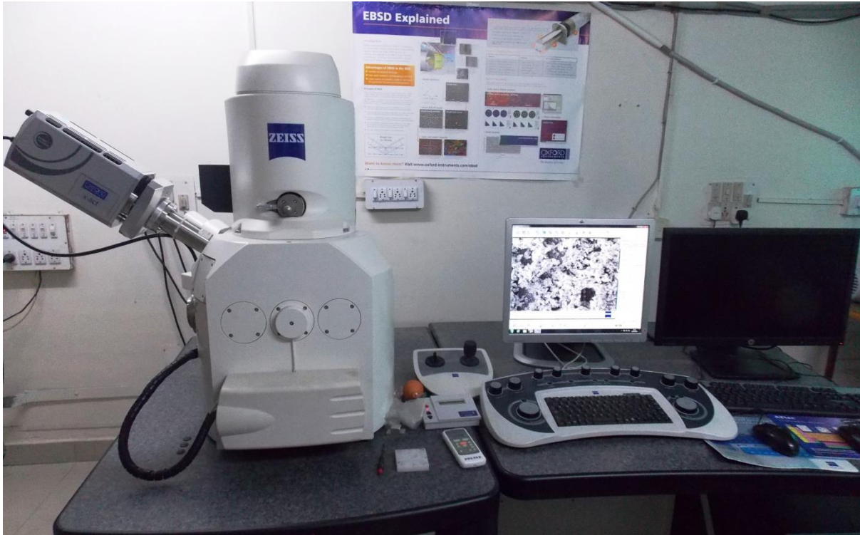
Fig.7. ZEISS scanning electron microscope used to observe the UFG microstructure
