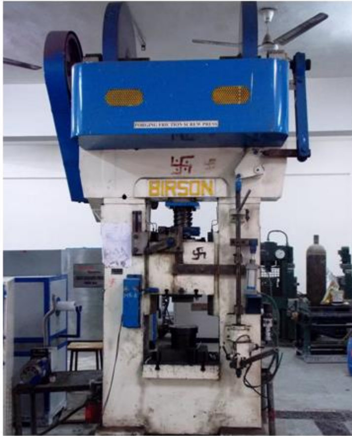
Fig.3. Forging press with open die used for multi-axial forging
