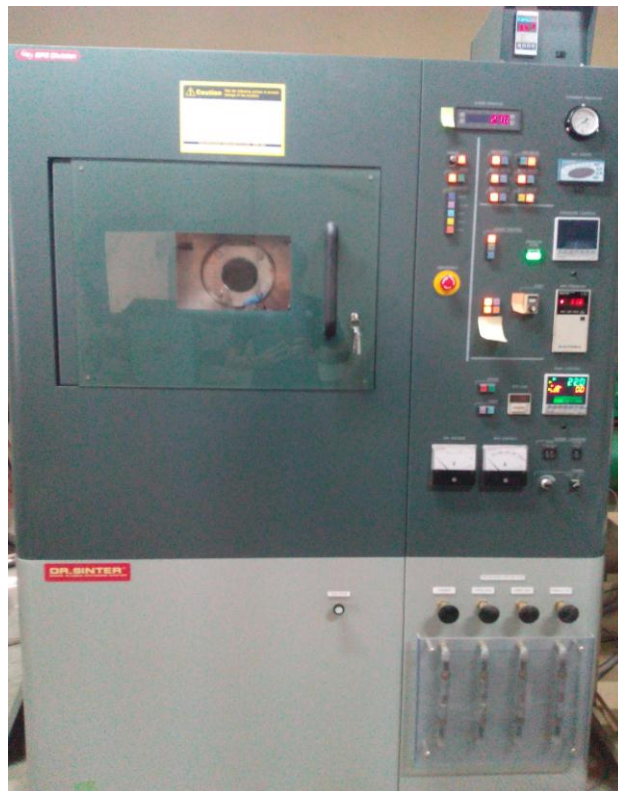
Fig. 3.2. Spark Plasma Sintering Machine
