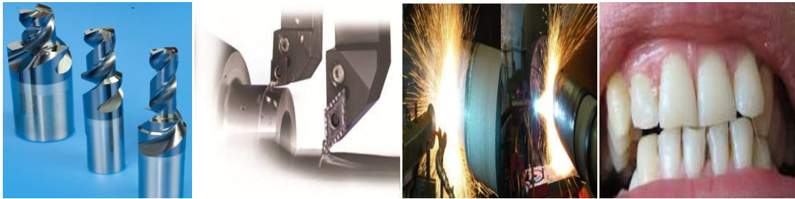
Fig. 2.2. Applications of TiCN-based cermets [ https://wikipedia.org/Titanium nitride ]
