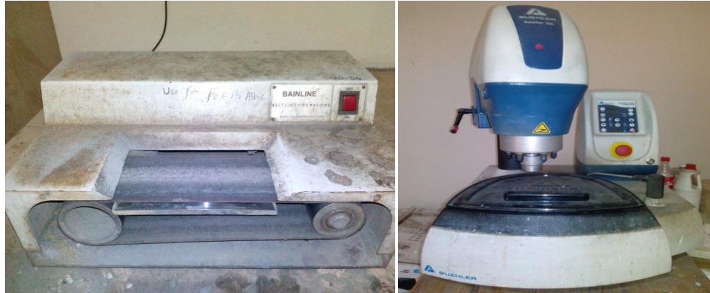
Fig. 3.3. (a) Belt Polishing Machine (b) Auto Polisher
