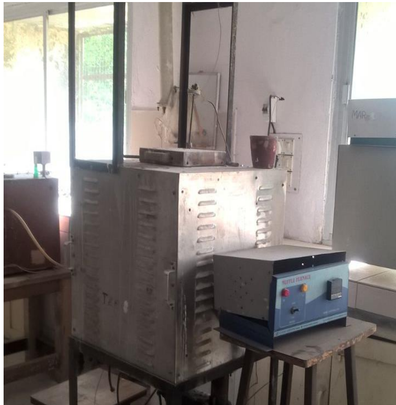
Fig. 7 Furnace used for the casting of in-situ Al composites.
