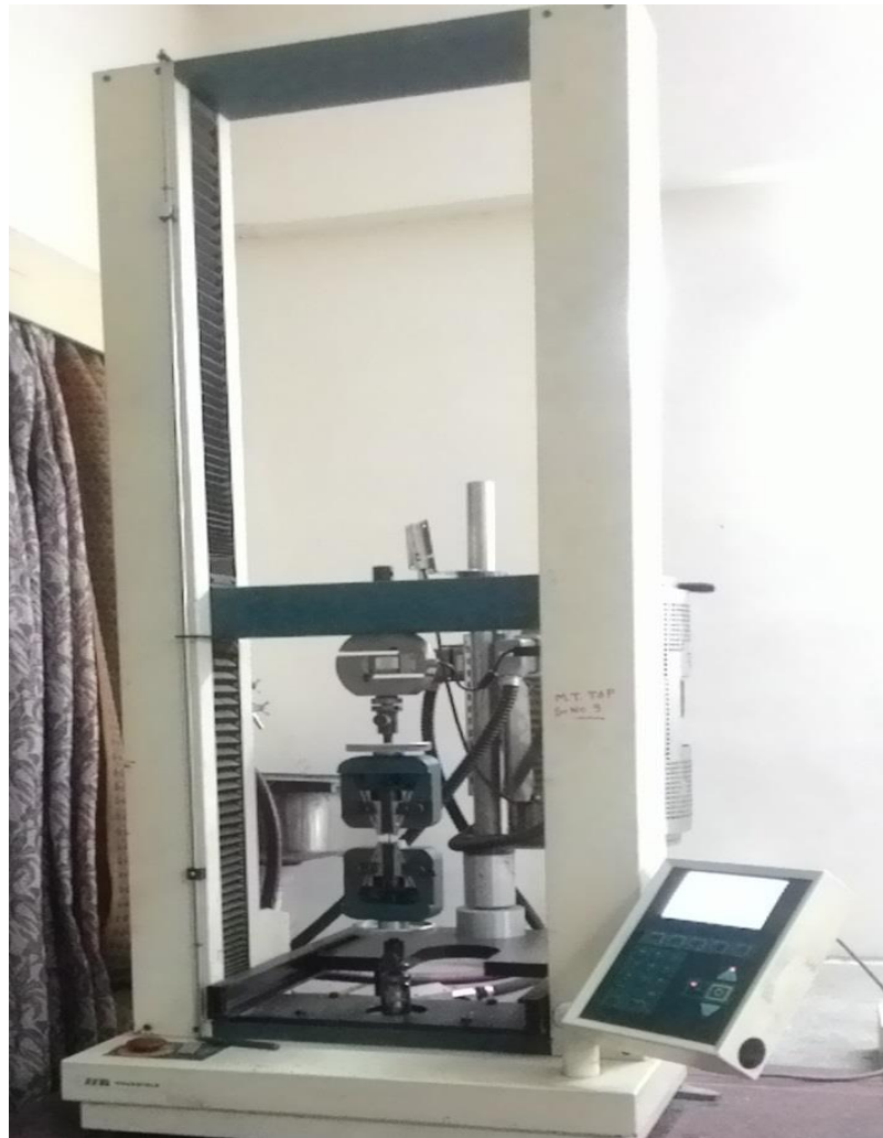
Fig. 10 Universal Testing Machine Model H-75 KS for tensile testing
