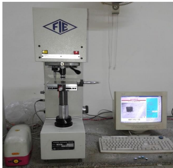
Fig. 11 Computerized Vickers Hardness Tester in MMED, IIT Roorkee
