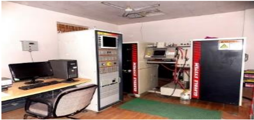
Fig. 14 Gleeble-3800 thermo mechanical-simulation facility in Materials and Metallurgy department, IIT Roorkee
