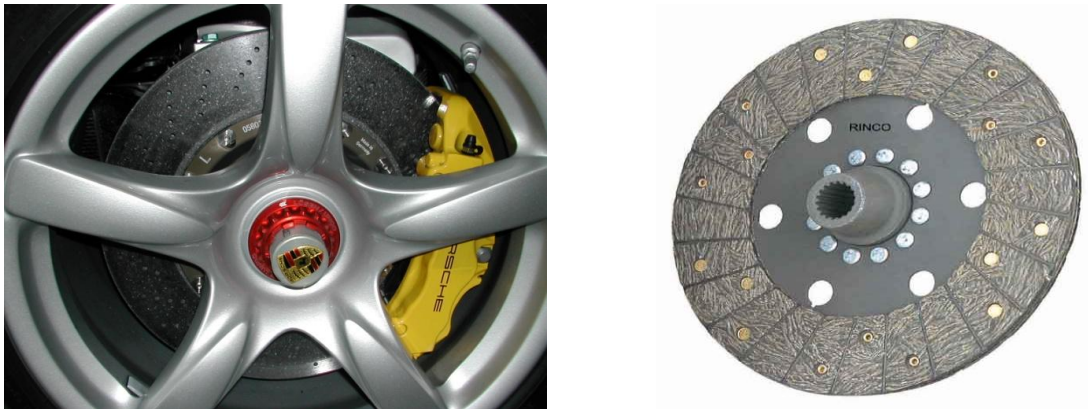
Fig. 2.5 Disc brake and clutch plate made of silicon carbide [39].
