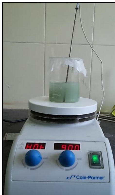
Fig.3.4. Photograph of Leaching setup.
