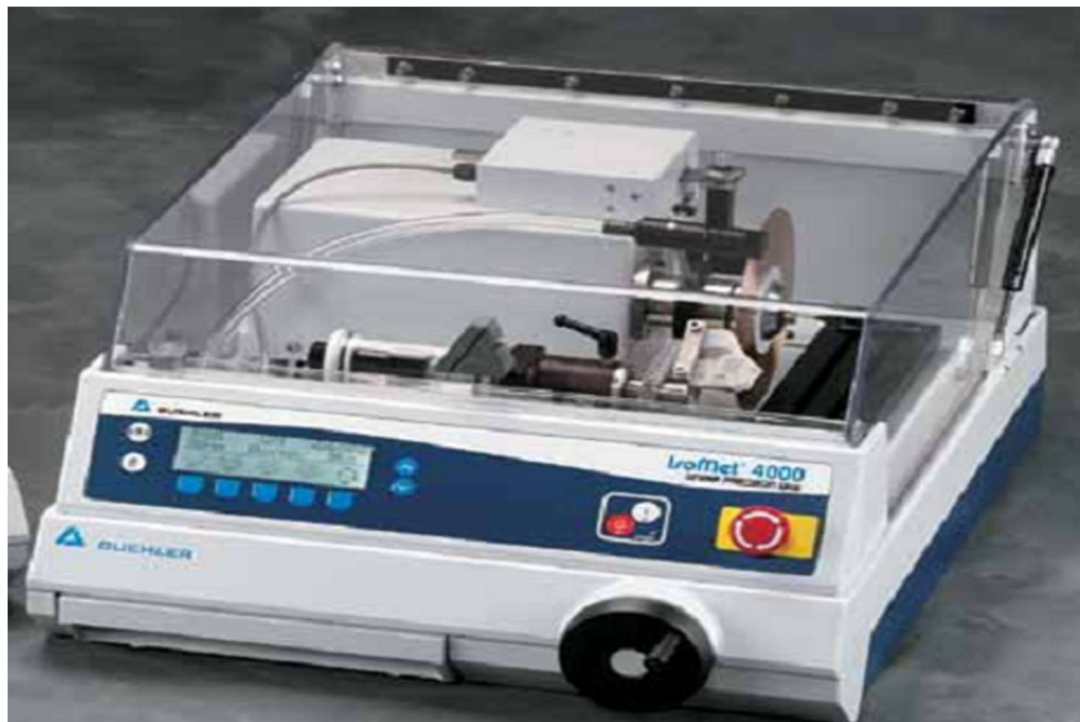
Fig. 3.7. High speed diamond saw "IsoMet 4000".
