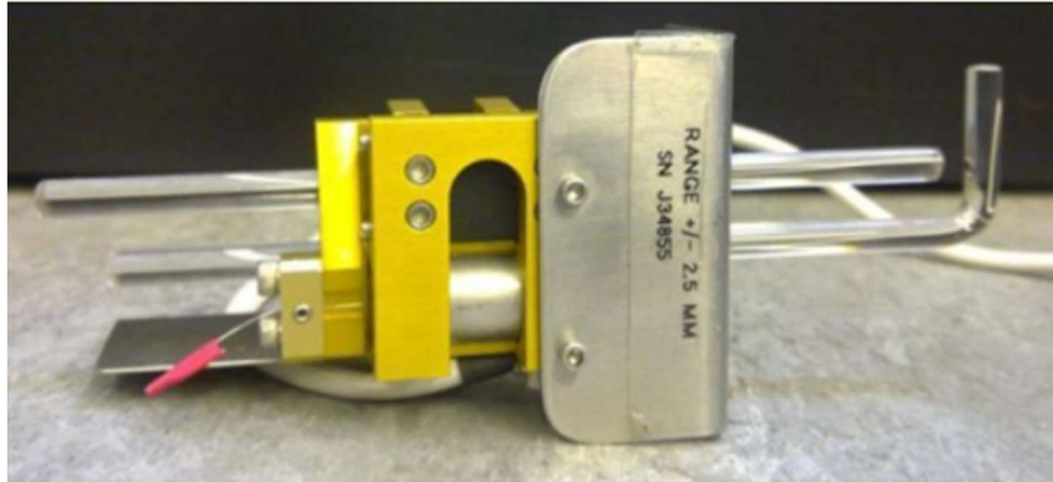
Fig. 3.2. LVDT dilatometer with a range of \pm 2.5 mm.
