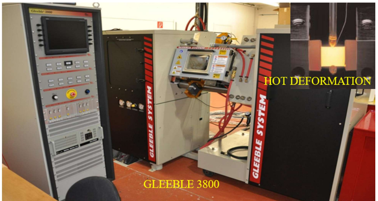
Fig. 3.5. Hot deformation under Gleeble ® 3800 thermomechanical simulator.
