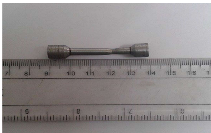
Fig. 5.2. Image of specimen after tensile test.
