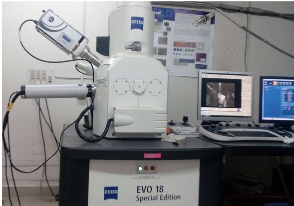
Fig. 3.8. Photograph of EVO 18 Zeiss scanning electron microscope.
