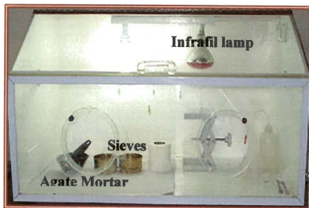
Fig. II.1 Dust free chamber for sample preparation
