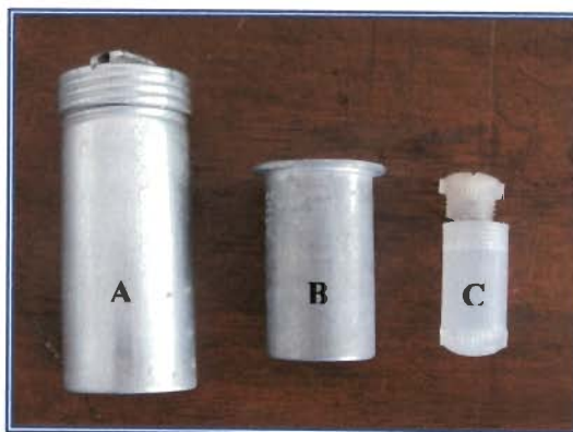
Fig. II.2 Irradiation containers for (A) CIRUS, (B) Dhruva and (C) Rabbit for Dhruva PCF
