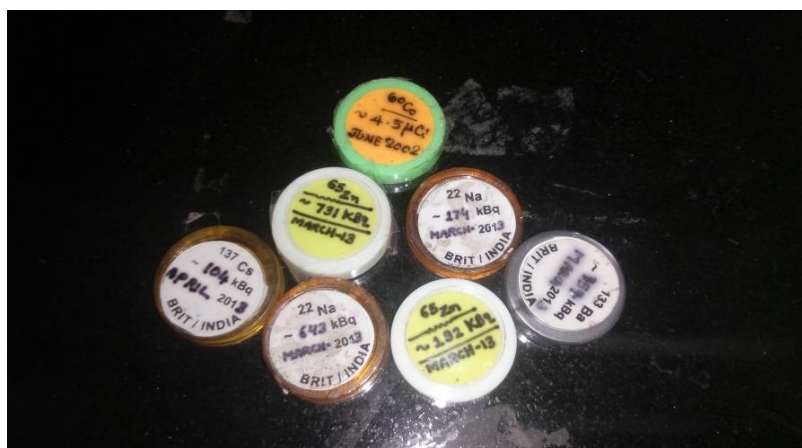
Figure 4.9 Different radioactive gamma sources
