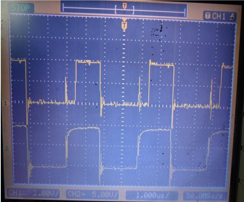
Figure 5.16 Deadband circuit input and output waveforms
