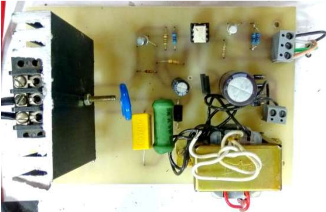
Figure 5.6 Image of the switch driver circuit
